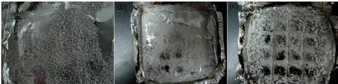
**Figure 8.** Photographs of residues for composites PP-5%LDH, PP-10%LDH and PP-20%LDH after cone calorimeter testing; (a) PP-5%LDH; (b) PP-10%LDH; and (c) PP-20%LDH.
