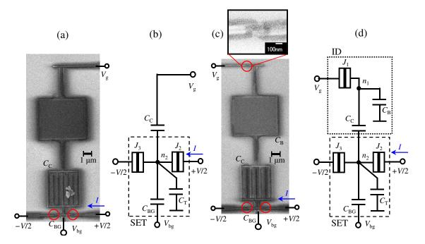
**Figure 1.** (a) Scanning electron microscope (SEM) image of a single electron transistor (SET) without an input discretizer (ID). Red circles indicate tunnel junctions; (b) The equivalent circuit of the SET without the ID; (c) The SEM image of the SET with the ID. The inset shows a close-up the tunnel junction of  $J_1$ ; (d) The equivalent circuit of the SET with the ID.
