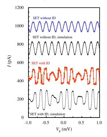
**Figure 3.** *I*-*V*<sub>g</sub> for input-output characteristics. Crossed marks, open squares and two solid lines correspond the SET without the ID at  $V = 78 \,\mu\text{V}$ , the SET with the ID at  $V = 74 \,\mu\text{V}$  and the best fits using a numerical simulation, respectively. Curves are vertically shifted by 250 pA for clarity.
