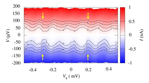
**Figure 2.** Current *I* characteristics of the SET with the ID as a function of *V* and  $V_g$  for  $V_{bg} = 0$  V at T < 80 mK. Borders of contour lines are plotted of 0.1, 0.2, 0.3, 0.4, -0.1, -0.2, -0.3 and -0.4 nA. Abrupt modulation of *I* against  $V_g$  are indicated by yellow arrows.
