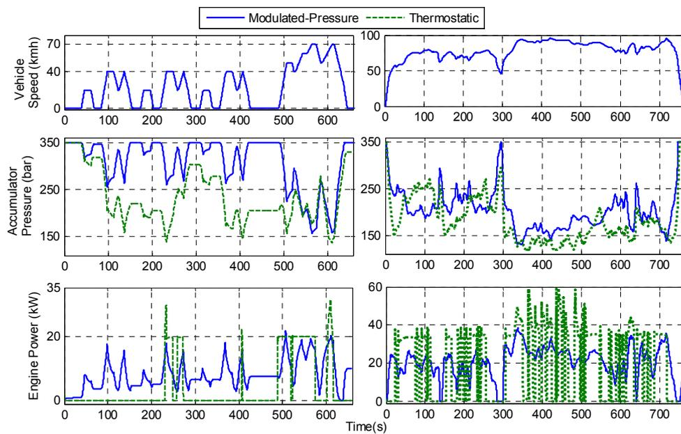
Figure 15. Modulated-Pressure and Thermostatic Control Strategies Comparison.
