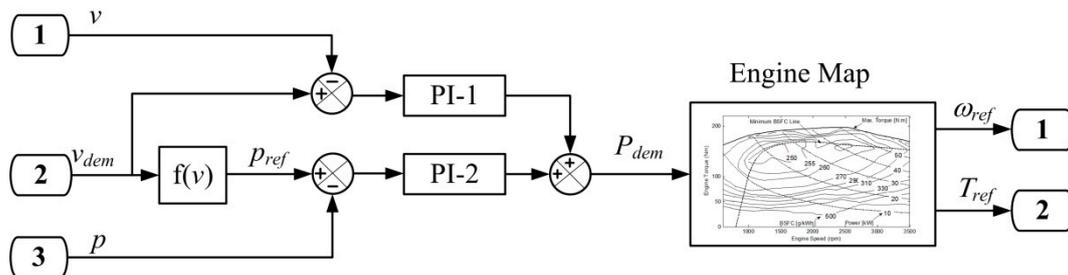
Figure 6. Schematic of Modulated-Pressure Control Strategy.
