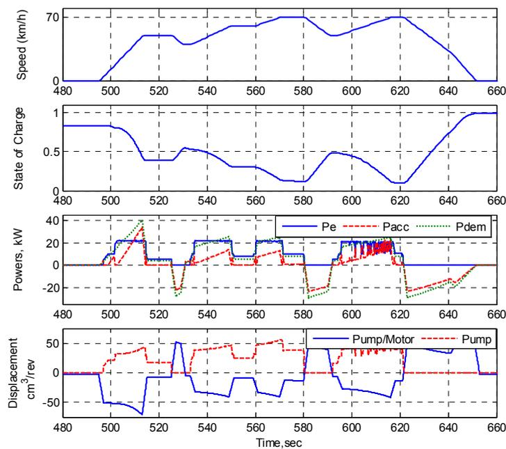
Figure 12. System Behaviors during 480–660 s Intervals of Japan 1015 Driving Cycle.
