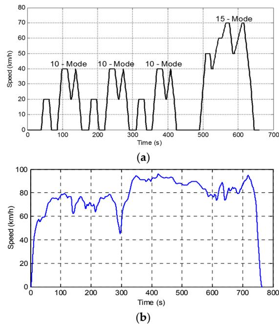
**Figure 3.** Velocity Reference Trajectories. (a) Japan 1015 Driving Cycle; (b) Highway Fuel Economy Test Driving Cycle.
