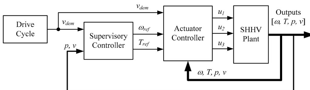
**Figure 4.** Hierarchical Control System of the SHHV.
