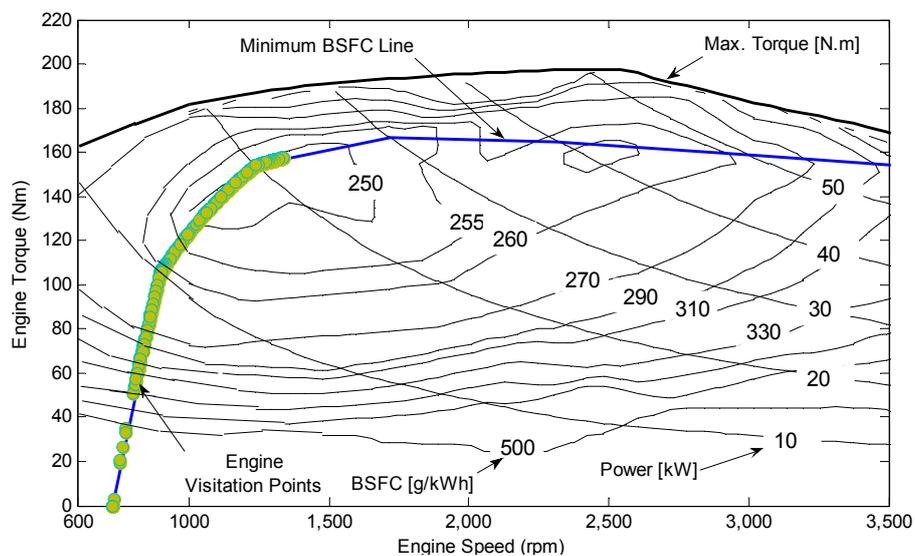
Figure 14. Engine Visitation Points under Japan 1015 Driving Cycle.
