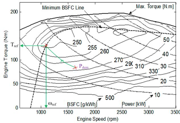
Figure 9. Engine Torque and Engine Speed Estimation.
