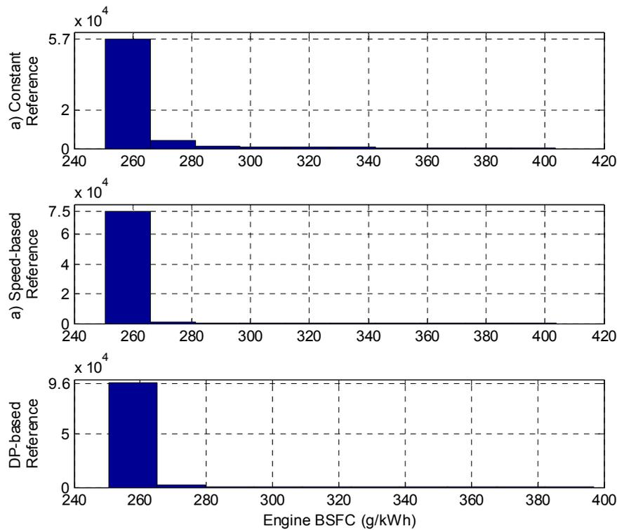
Figure 18. Number of Occurrence of Engine Operating Points on BSFC map.
