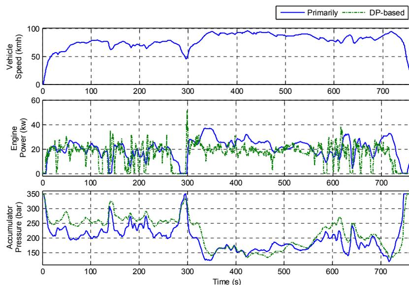
Figure 17. Pressure Trajectories with Primary and DP-Based Modulated-Pressure Strategies.
