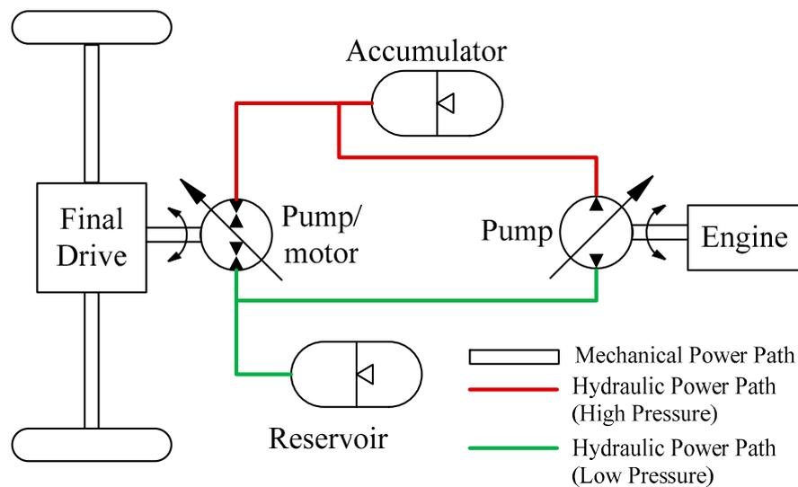
**Figure 1.** Schematic and Control Signal Paths of Series Hydraulic Hybrid Vehicle (SHHV).
