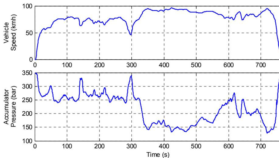
Figure 13. Accumulator Pressure Trajectory under Highway Fuel Economy Test (HWFET).
