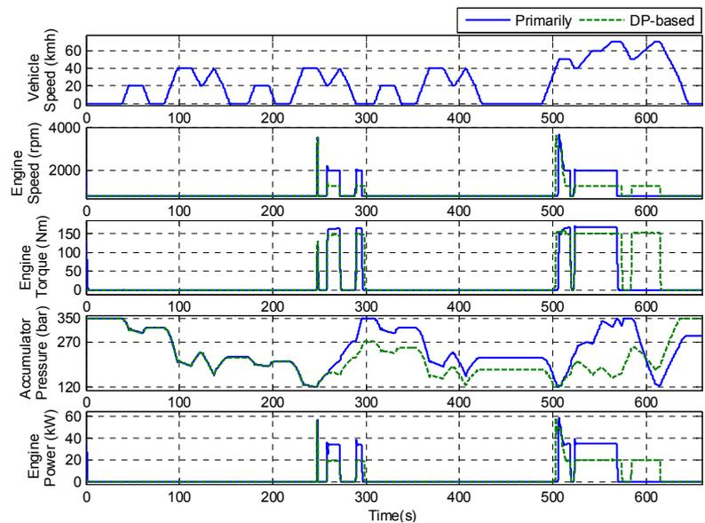
Figure 16. Pressure Trajectories with Primary and DP-Based Thermostatic.
