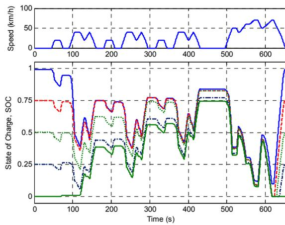
Figure 10. State-of-Charge (SOC) Trajectories with Different Initial Condition.
