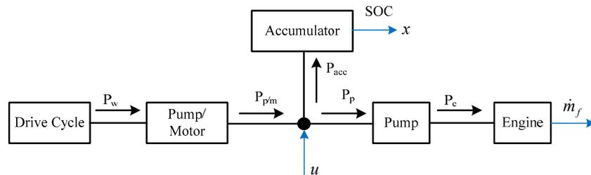
Figure 8. Backward Model of the SHHV.
