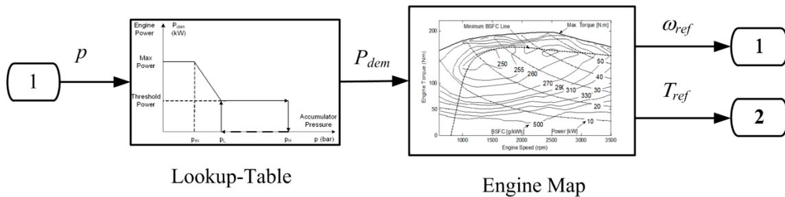
Figure 5. Schematic of Thermostatic Control Scheme.
