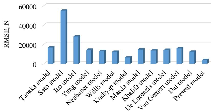
Figure 5. Comparison of GEP model with existing methods in the prediction of the debonding force for the testing data.
