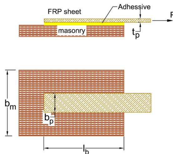
Figure 1. Adhesive-bonded joint [24].
