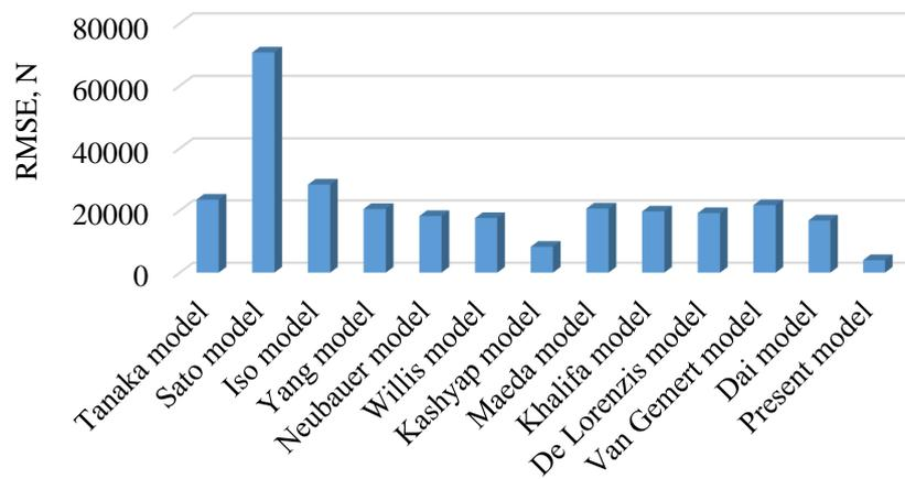
Figure 4. Comparison of the GEP model with existing methods in the prediction of the debonding force for the training data.
