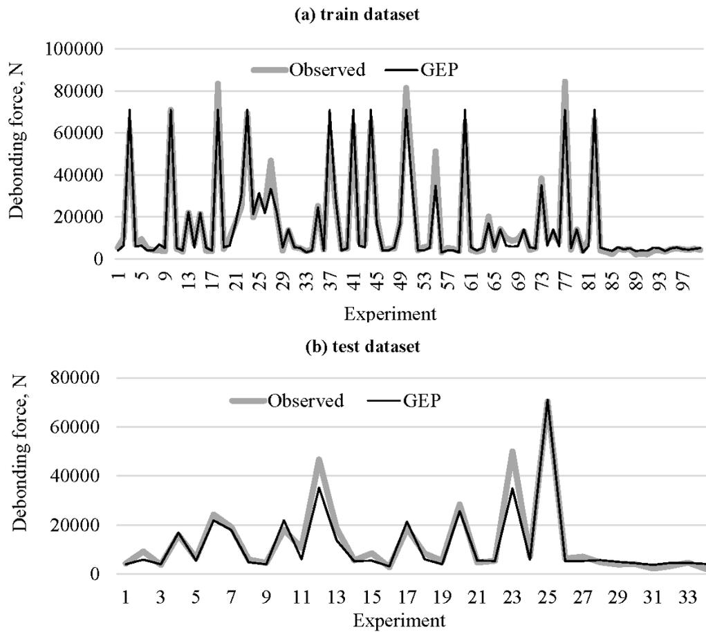
**Figure 2.** Observed and predicted debonding forces by GEP (gene expression programming) for (a) training dataset and (b) testing dataset.
