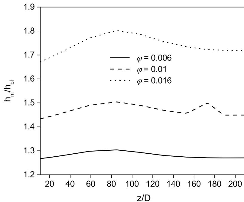
**Figure 8.** Axial variations of the heat transfer coefficient ratio  $h_{nf}/h_{bf}$  for  $d_{np} = 42$  nm,  $Re = 1600$  and three volume fractions in  $Al_2O_3$  nanoparticles:  $\phi = 0.006$ ,  $0.01$  and  $0.016$ .
