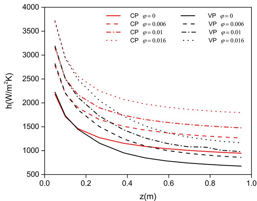
**Figure 6.** Local heat transfer coefficient obtained for  $Re = 1600$ ,  $d_{np} = 42$  nm and  $Al_2O_3$ -water based nanofluids: Influence of temperature-dependent properties on the performances of the mixture model.
