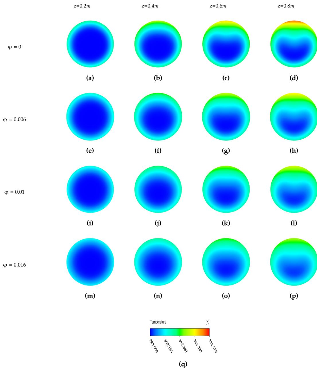
**Figure 9.** Maps of temperature  $T$  at four axial positions:  $z = 0.2$  m (a,e,i,m);  $z = 0.4$  m (b,f,j,n);  $z = 0.6$  m (c,g,k,o); and  $z = 0.8$  m (d,h,l,p). Results obtained for  $d_{np} = 42$  nm,  $Re = 1600$  and four volume fractions of  $Al_2O_3$  nanoparticles:  $\varphi = 0$  (a–d); 0.006 (e–h); 0.01 (i–l); and 0.016 (m–p).
