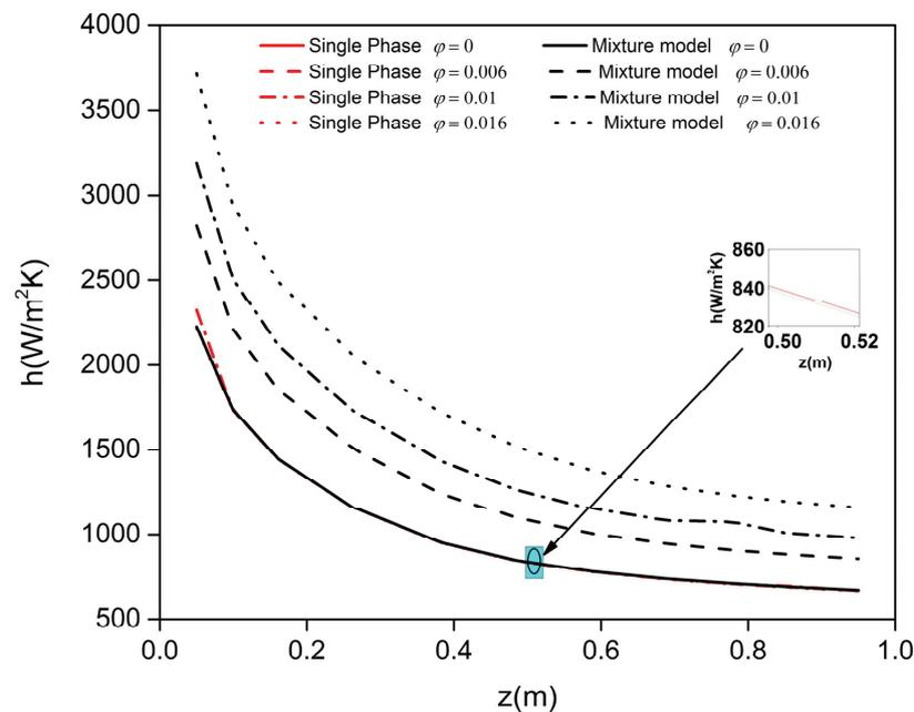
**Figure 5.** Local heat transfer coefficient obtained for  $Re = 1600$ ,  $d_{np} = 42$  nm and  $Al_2O_3$ -water based nanofluids: comparison between the single-phase and mixture models with temperature-dependent properties.
