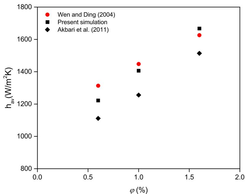
**Figure 4.** Influence of the concentration of  $Al_2O_3$  nanoparticles  $\varphi$  on the average heat transfer coefficient for  $Re = 1600$  and  $d_{np} = 42$  nm. Comparisons with the experimental data of Wen and Ding [11] and the numerical simulations of Akbari et al. [19].
