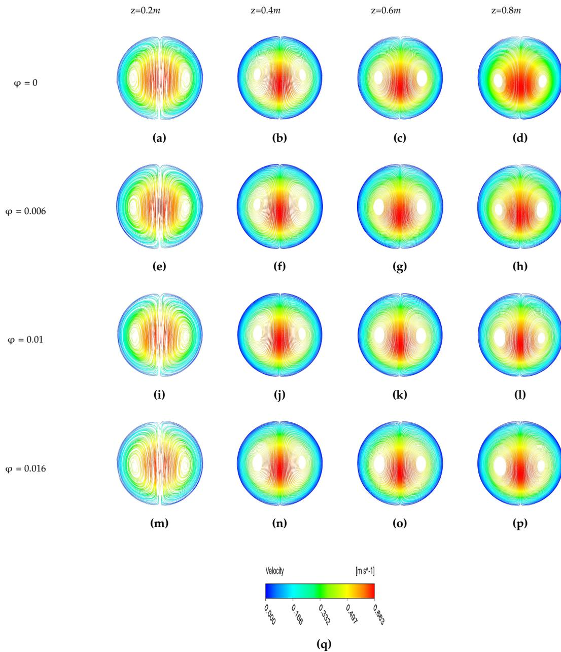
**Figure 10.** Streamline patterns colored by the axial velocity component  $w$  at four axial positions:  $z = 0.2$  m (a,e,i,m);  $z = 0.4$  m (b,f,j,n);  $z = 0.6$  m (c,g,k,o); and  $z = 0.8$  m (d,h,l,p). Results obtained for  $d_{np} = 42$  nm,  $Re = 1600$  and four concentrations of  $Al_2O_3$  nanoparticles:  $\varphi = 0$  (a–d); 0.006 (e–h); 0.01 (i–l); and 0.016 (m–p).
