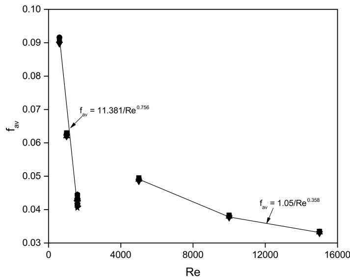
**Figure 16.** Influence of the Reynolds number  $Re$  on the average friction coefficient  $f_{av}$ . Results obtained for all values of  $\varphi$ ,  $d_{np}$  and all types of nanofluids.
