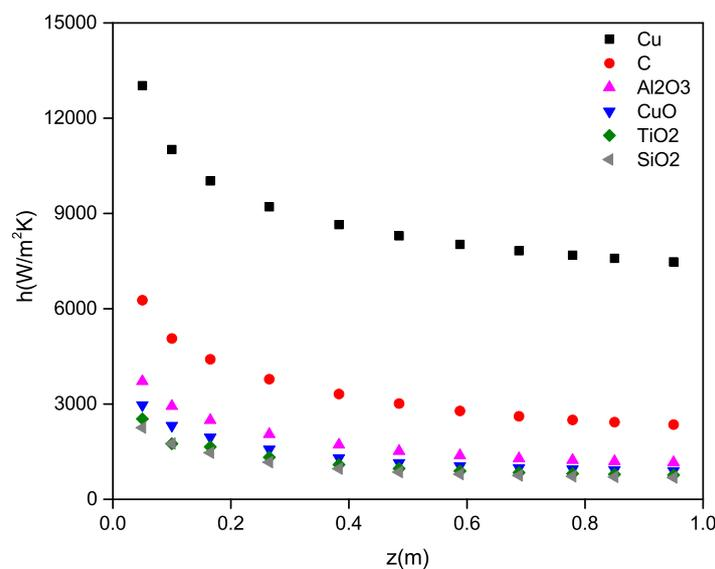
**Figure 14.** Axial variations of the local heat transfer coefficient  $h$  for six types of nanoparticles with  $d_{np} = 42$  nm,  $\phi = 0.016$  and  $Re = 1600$ .
