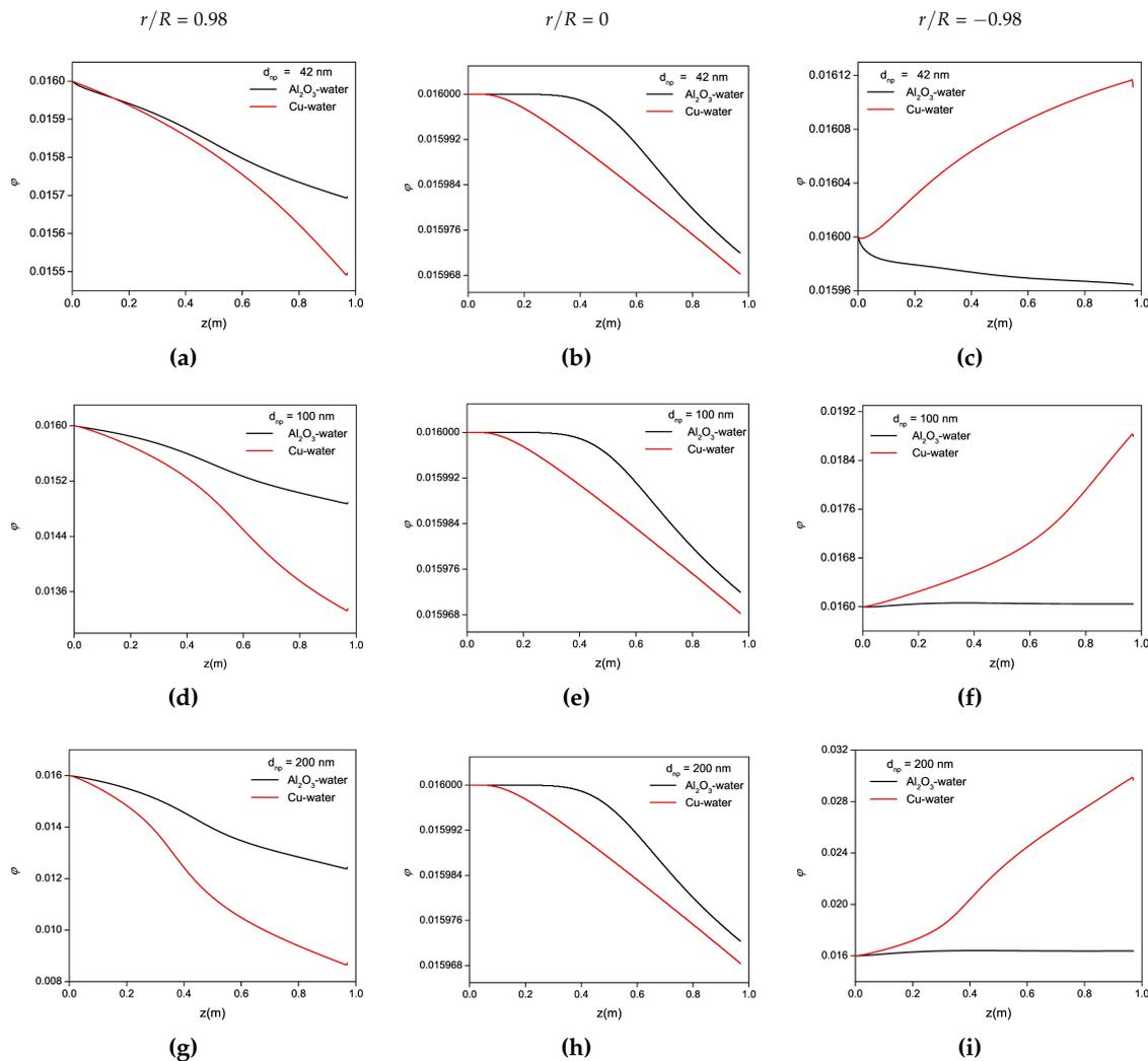
**Figure 12.** Axial variations of the volume fraction  $\phi$  at three radial locations:  $r/R = 0.98$  (a,d,g);  $r/R = 0$  (b,e,h); and  $r/R = -0.98$  (c,f,i). Results obtained for Cu and  $Al_2O_3$  nanoparticles of three different diameters  $d_{np} = 42$  nm (a–c); 100 nm (d–f); and 200 nm (g–i) with  $\phi = 0.016$  and  $Re = 1600$ .
