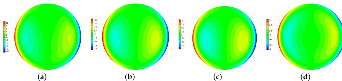
**Figure 11.** Contours of the streamwise vorticity at  $z = 0.8$  m: (a)  $\varphi = 0$ ; (b)  $\varphi = 0.006$ ; (c)  $\varphi = 0.01$ ; and (d)  $\varphi = 0.016$ . Results obtained for  $d_{np} = 42$  nm,  $Re = 1600$  and  $Al_2O_3$  nanoparticles.
