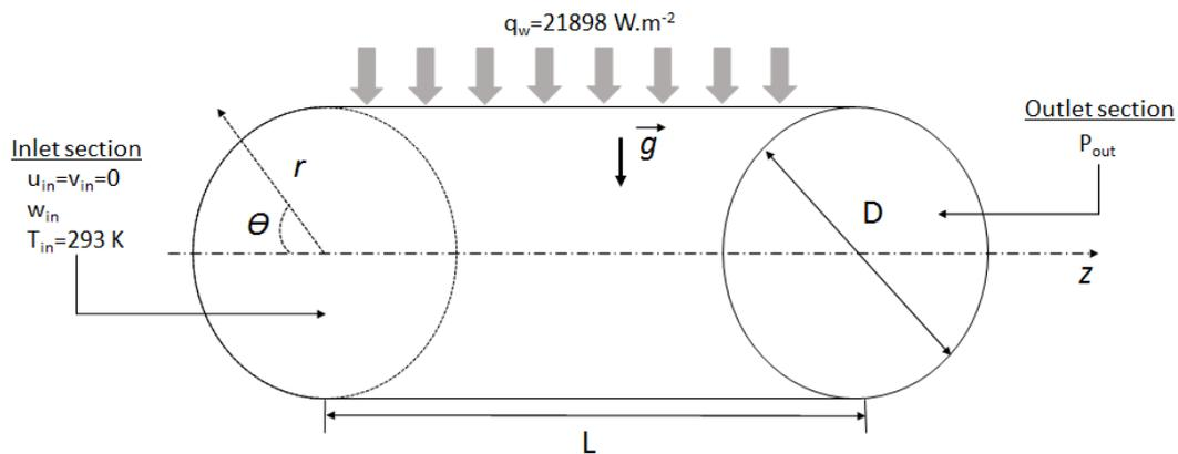
Figure 1. Schematic view of the computational domain with the boundary conditions.
