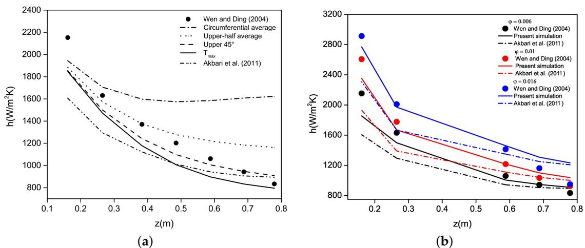
**Figure 3.** Axial variations of the local heat transfer coefficient  $h(z)$  predicted by the mixture model for  $Al_2O_3$  water-based nanofluids: (a) different methods for the evaluation of the wall temperature  $T_w$  for  $\varphi = 0.006$ ; (b) three nanoparticle concentrations ( $\varphi = 0.006, 0.01$  and  $0.016$ ). Comparisons for  $Re = 1600$  and  $d_{np} = 42$  nm with the experimental data of Wen and Ding [11] and the numerical simulations of Akbari et al. [19].
