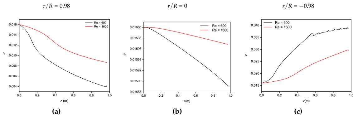
**Figure 13.** Axial variations of the volume fraction  $\phi$  in Cu nanoparticles at three radial locations: (a)  $r/R = 0.98$ ; (b)  $r/R = 0$ ; and (c)  $r/R = -0.98$ . Results obtained for Cu nanoparticles of diameter  $d_{np} = 200$  nm with  $\phi = 0.016$  and two Reynolds numbers  $Re = 600$  and  $1600$ .
