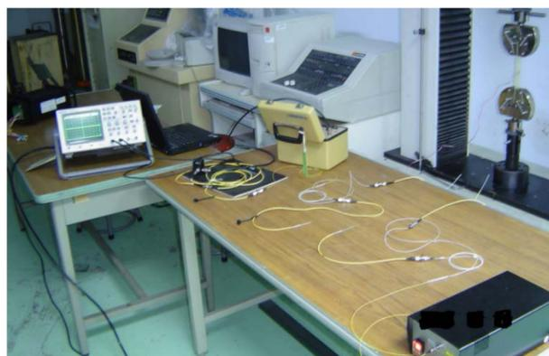
Figure 3. Experimental setup of the tensile test measured by Mach–Zehnder interferometry.
