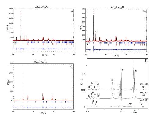
**Figure 7.** X-ray diffractograms corresponding to (a) x = 0.09; (b) x = 0.13; (c) x = 0.17; (d) diffractograms presenting the dependence of intensity (I) on interplanar distances (d) and Ce concentration (*x*). The vertical bars correspond to the monoclinic (M) and tetragonal (T) phases (FullProf program was used for determination of parameters). SP represents the foreign phase.
