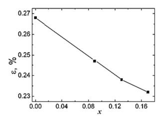
**Figure 5.** The dependency of microstrain,  $\varepsilon$ , on the concentration of Ce ions (*x*).
