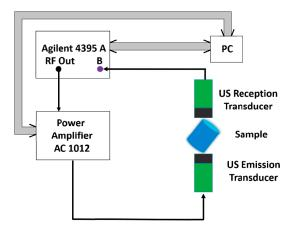
**Figure 1.** RUS Experimental setup schematic block diagram. Thin lines correspond to coaxial cable for sinusoidal wave transmission; thick lines are GPIB cable for digitalized data.
