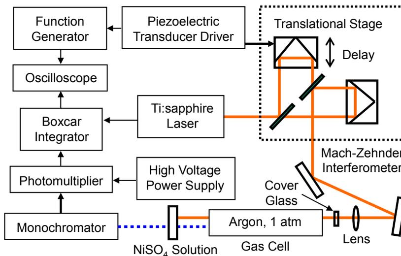
**Figure 1.** Experimental apparatus for third harmonic generation-fringe-resolved autocorrelator (THG-FRAC). The orange (solid) and blue (broken) lines show the fundamental and THG beams, respectively.
