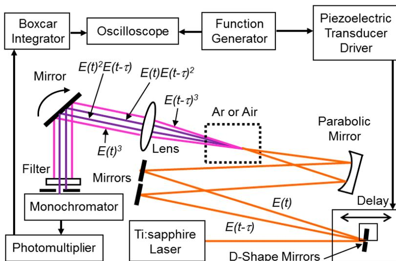
**Figure 2.** Experimental apparatus for THG-frequency-resolved optical gating (FROG).
