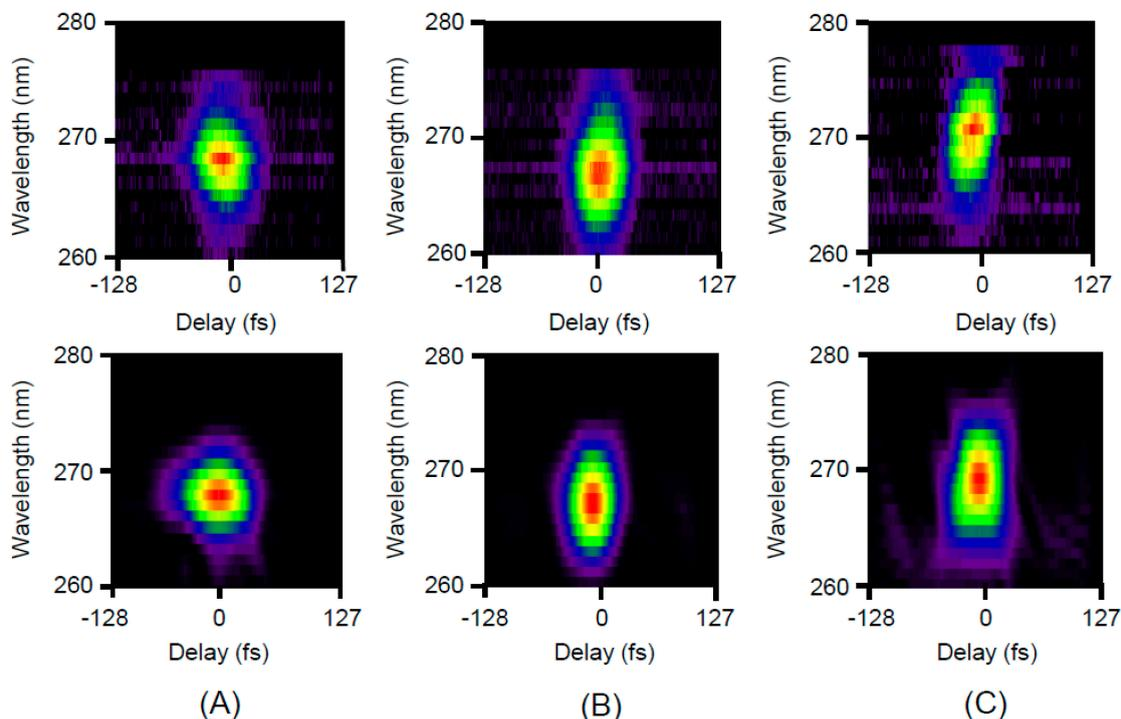
**Figure 5.** THG-FROG traces obtained for (A) negatively-chirped (B) FTL (C) positively-chirped pulses. The chirp of the pulse was adjusted by changing the position of the grating in the compressor of the Ti:sapphire laser to the value, at which the energy of the THG pulse decreased to a half of the value obtained using the FTL pulse. Above, original traces; below, retrieved data. FROG error: (A) 0.6% (B) 0.6% (C) 1%.
