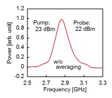
Figure 4 shows the dependence of the BGS on probe power when the pump power was fixed at 23 dBm. The probe power was reduced from 22 dBm down to 6 dBm, and averaging was conducted 30 times for the observable readout when the Stokes power was very low. As the probe power decreased, the Stokes power also decreased, which proves that this BGS is caused by the interaction between the pump light and the probe light, *i.e.*, SBS.
