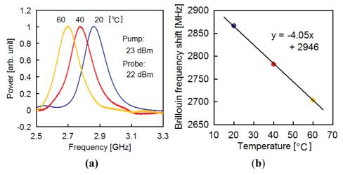
Figure 5. Dependence of (a) BGS and (b) BFS on temperature in PFGI-POF.
