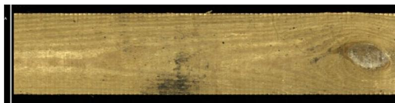
**Figure 4.** An image of a board that is dirty and has a knot, as well as a rough surface.
