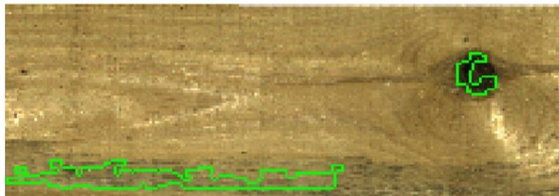
**Figure 12.** An image of a plank with the green outlines of defects marked.
