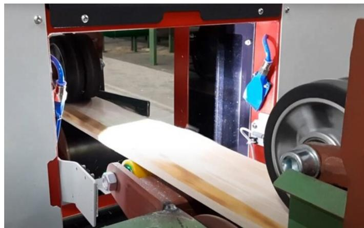
**Figure 2.** The working area of the vision system equipped with four sets of cameras and an illuminator, recording four sides of the board.
