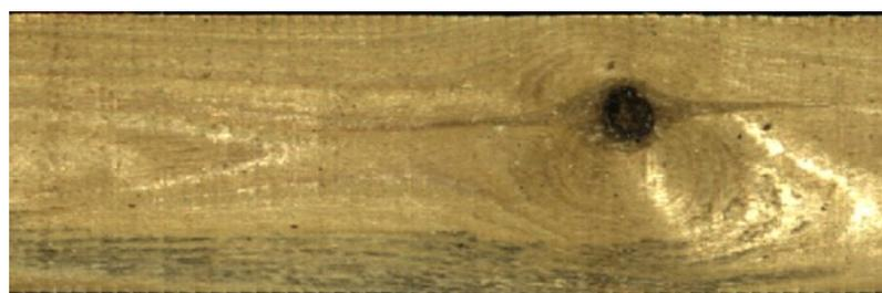
**Figure 10.** An image of a wood surface with a visible defect in the form of a blue stain and a knot.
