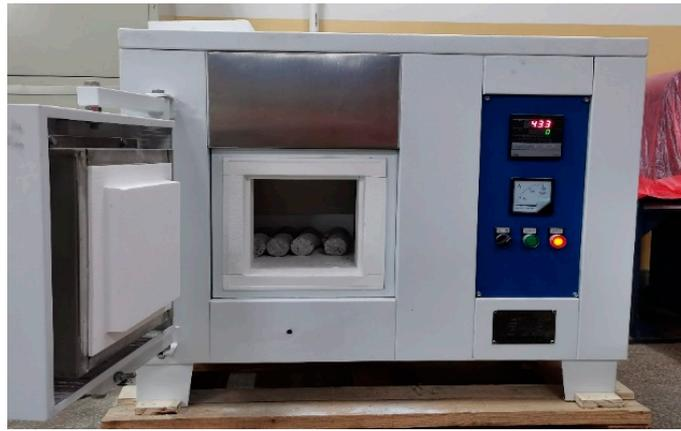
Figure 4. Electric resistance furnace chamber.
