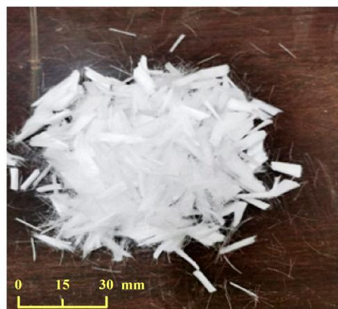
**Figure 2.** Polypropylene fiber.
