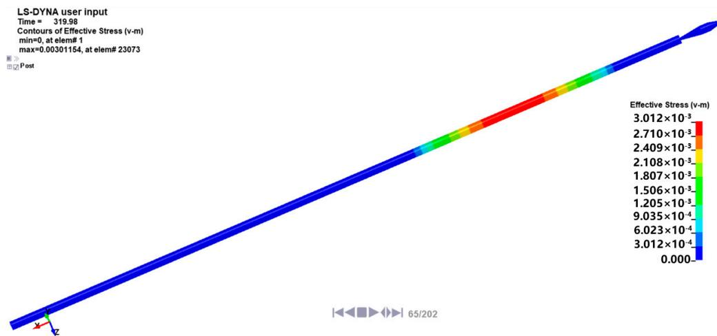
**Figure 19.** Propagation of the 360 stress  $\mu$ s wave.
