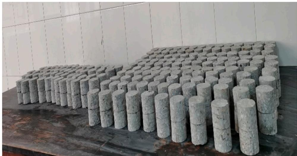
**Figure 3.** Prepared concrete specimens.
