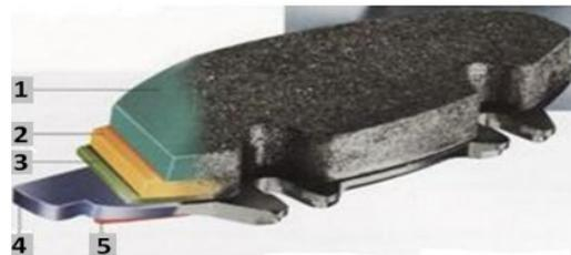
**Figure 2.** Brake pad: 1. friction material; 2. intermediate layer; 3. adhesive; 4. main frame; 5. damping layer.
