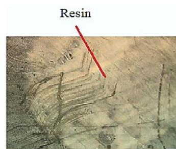
**Figure 3.** Resin film over brake pad analysis area.
