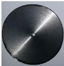
**Figure 5.** Brake disc sample polishing.
