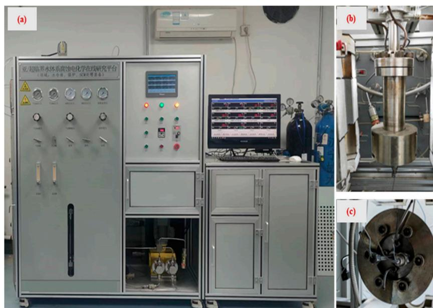
**Figure 14.** Photo show of a multi-functional sub-/supercritical water electrochemical research platform built in XJTU. (a) the main view of the research platform, (b) autoclave, (c) Reactor base and electrode arrangement.
