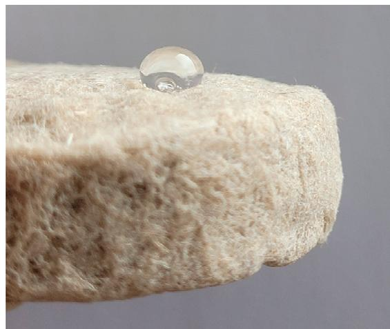
**Figure 2.** Determination of contact angle of aerogel.
