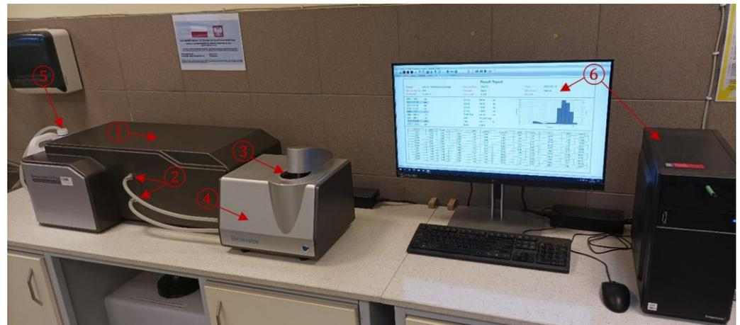
**Figure 7.** View of the Bettersizer S3 Plus laser particle size analyzer test stand located in the Department of Military Engineering and Infrastructure of the MUT, with markings of crucial components ①–⑥.
