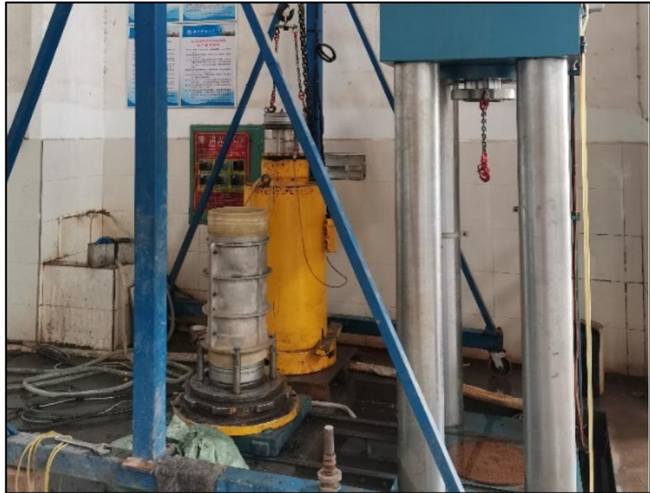
**Figure 3.** The large-scale dynamic and static triaxial instrument.
