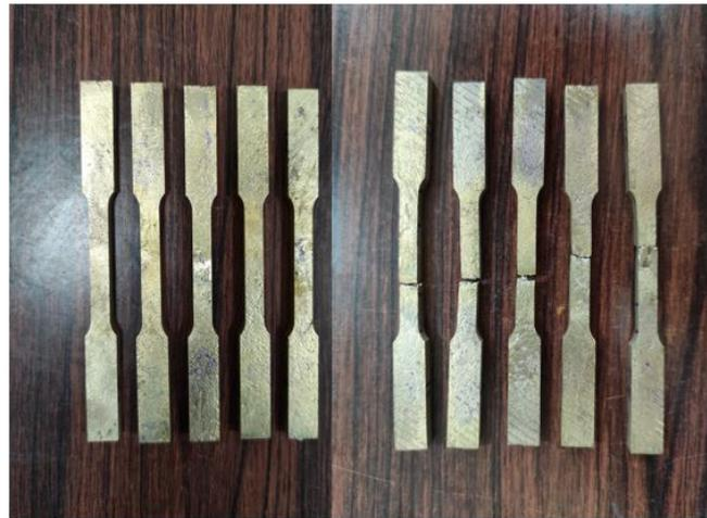
Figure 12. Tensile specimen before and after tensile test.
