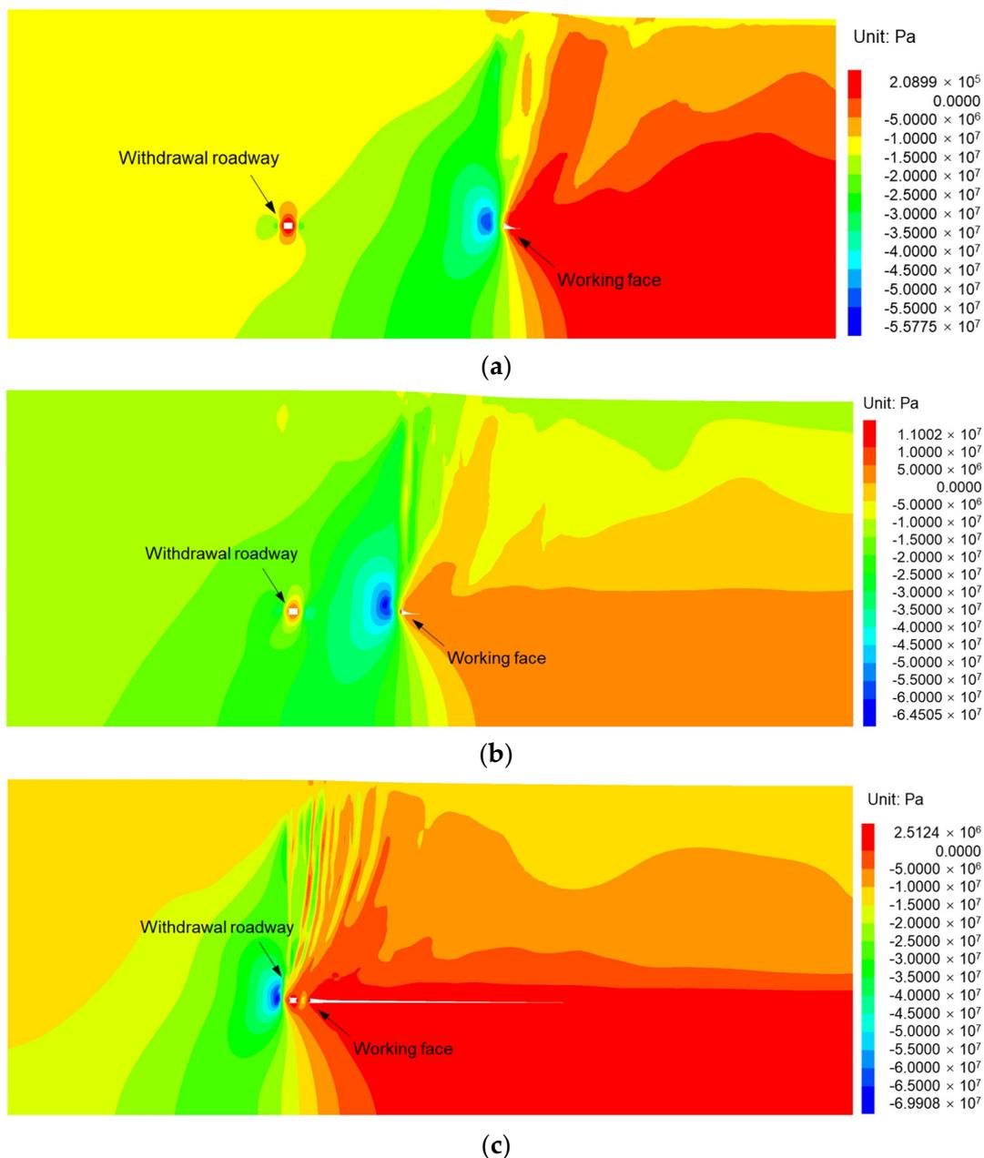
**Figure 6.** Vertical stress nephogram when the distance between the working face and the withdrawal roadway is (a) 115 m; (b) 55 m; (c) 5 m.
