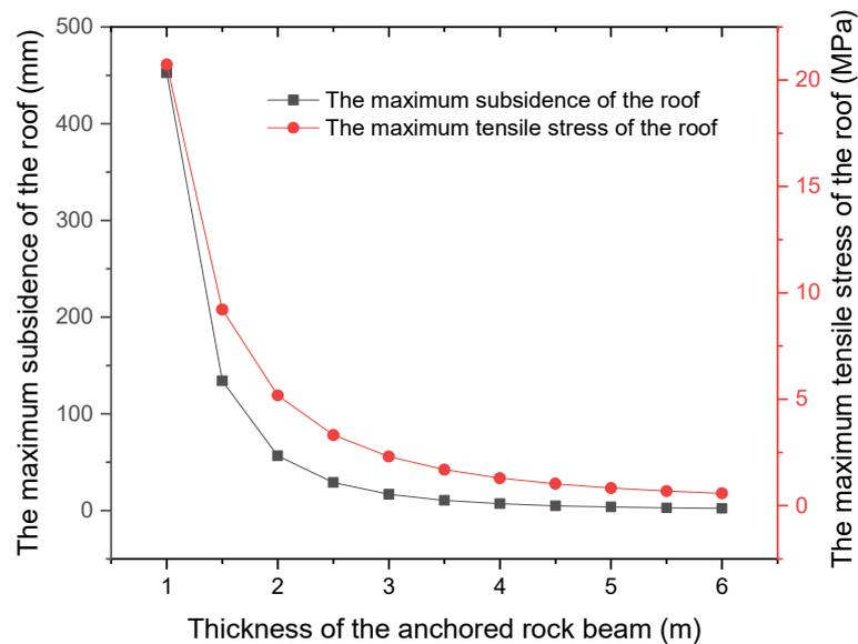
**Figure 8.** The relationship between the thickness of the anchored rock beam and the maximum subsidence/the maximum tensile stress of the roof.
