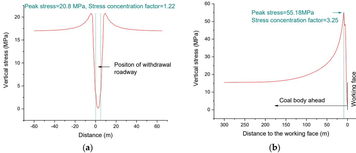
**Figure 4.** Distribution curve of abutment pressure: (a) The abutment pressure of coal mass on both sides of the withdrawal roadway; (b) Front abutment pressure of working face 21405.
