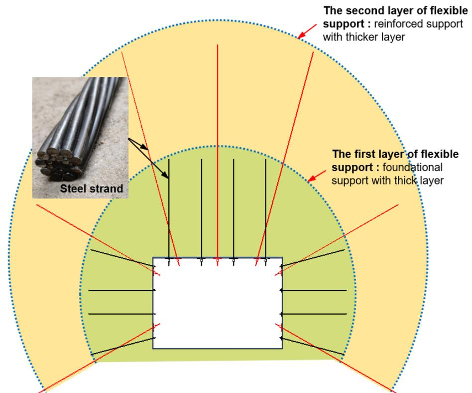
**Figure 9.** Supporting technique with double-layer flexible thick anchorage.
