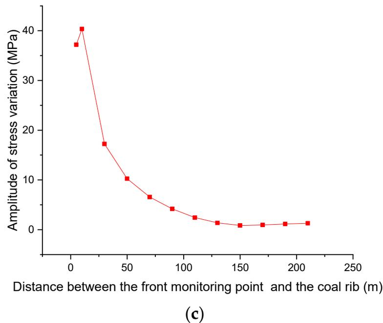
**Figure 7.** The evolution of vertical stress during mining: (a) The evolution curves of vertical stress at different measuring points in front of the working face; (b) The evolution curves of stress fluctuation value; (c) The amplitude of stress variation.
