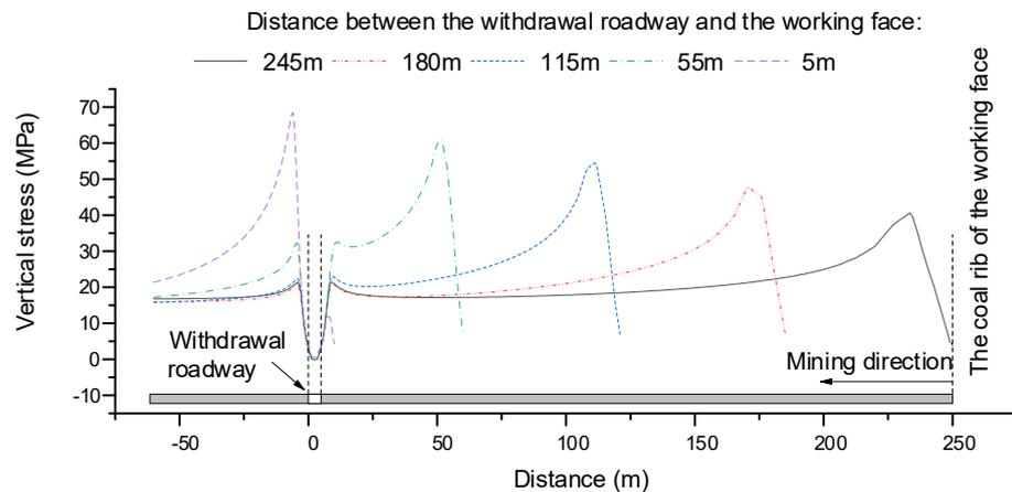
**Figure 5.** Vertical stress distribution curve at different distances between the working face and the withdrawal roadway.
