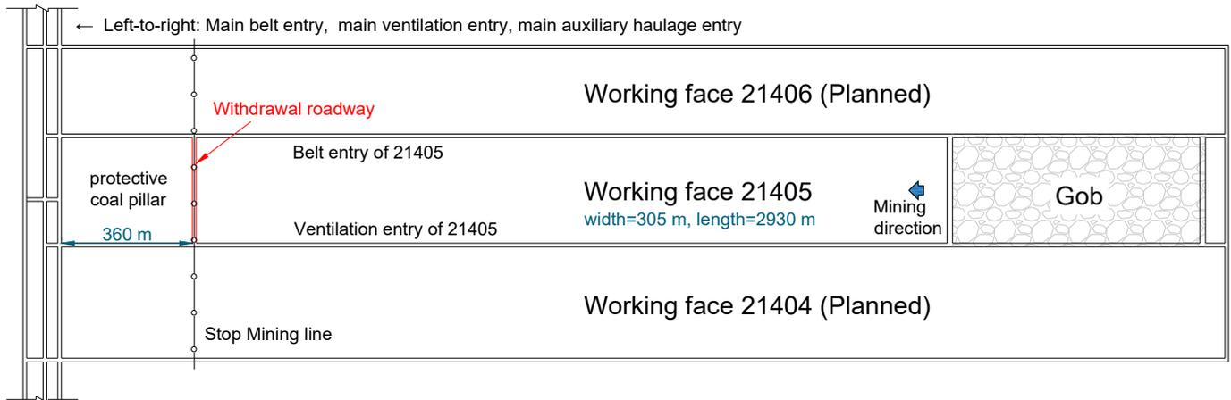
Figure 1. Roadway layout and mining environment.
