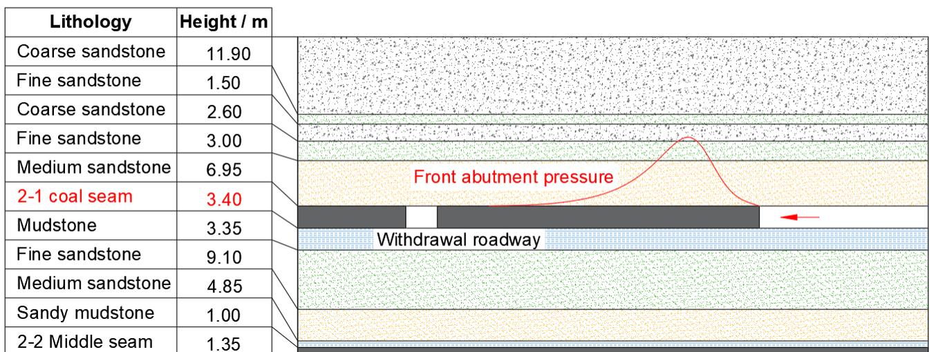
Figure 2. Profile view of the rock strata and the relationship between the withdrawal roadway and the working face.
