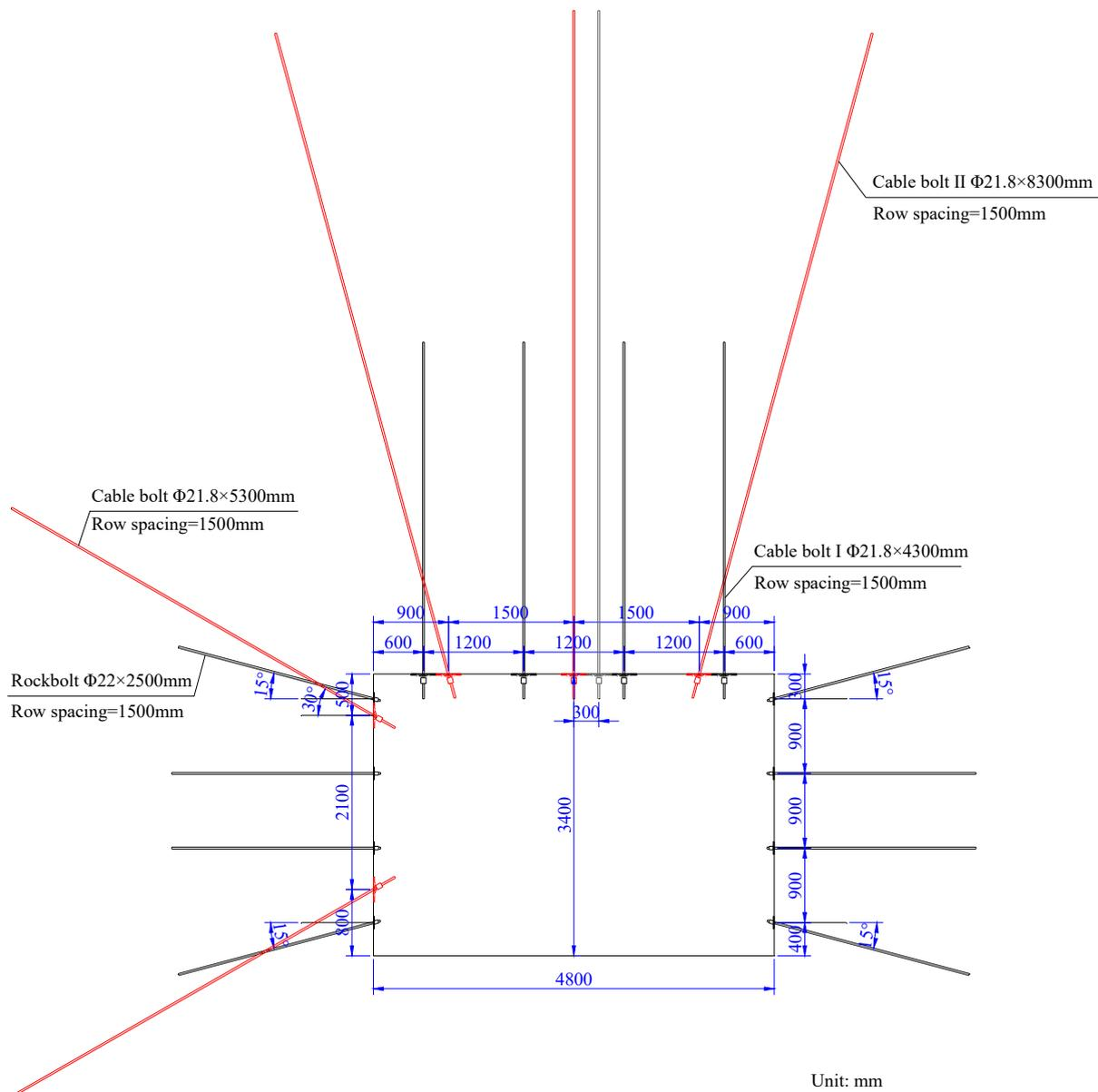
**Figure 10.** The support parameters of withdrawal roadway 21405.
