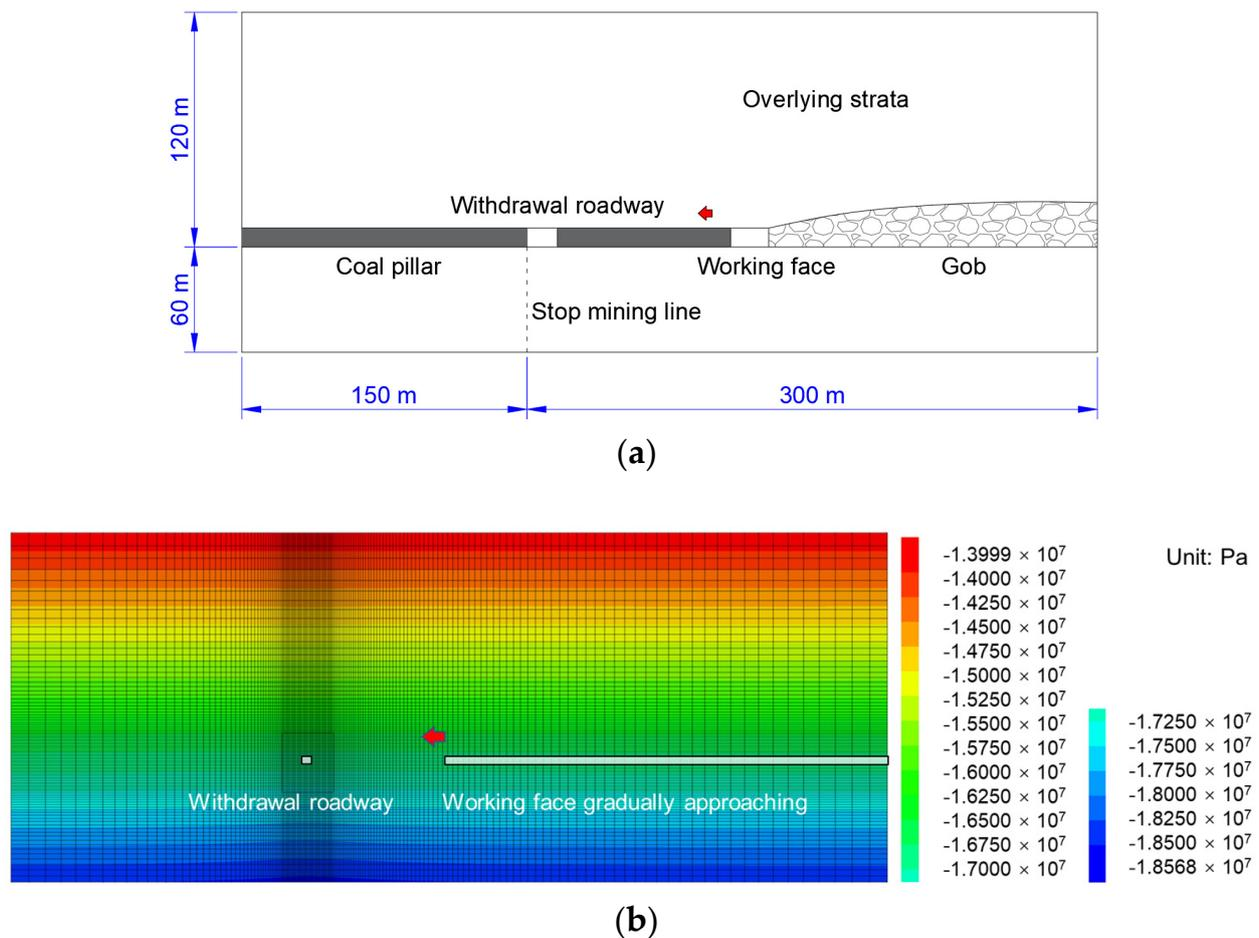
**Figure 3.** Numerical calculation model of the withdrawal roadway and the working face: (a) The spatial relationship and size of the model; (b) Numerical modeling and in situ stress field.
