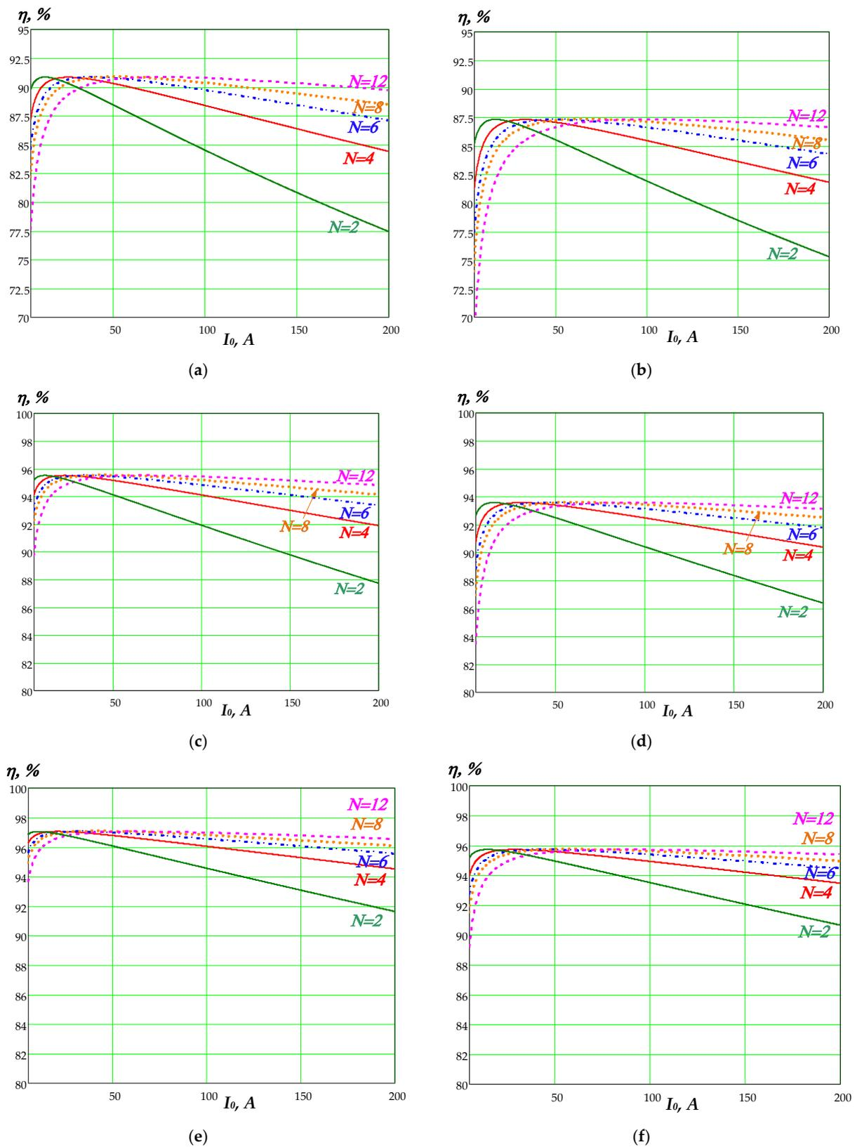
**Figure 3.** Multi-phase synchronous buck converter efficiency  $\eta$  vs. output current  $I_0$ : (a) Duty cycle  $D = 0.133$ ,  $f_{SW} = 200$  kHz; (b) duty cycle  $D = 0.133$ ,  $f_{SW} = 300$  kHz. (c) duty cycle  $D = 0.275$ ,  $f_{SW} = 200$  kHz; (d) duty cycle  $D = 0.275$ ,  $f_{SW} = 300$  kHz; (e) duty cycle  $D = 0.417$ ,  $f_{SW} = 200$  kHz; (f) duty cycle  $D = 0.417$ ,  $f_{SW} = 300$  kHz.
