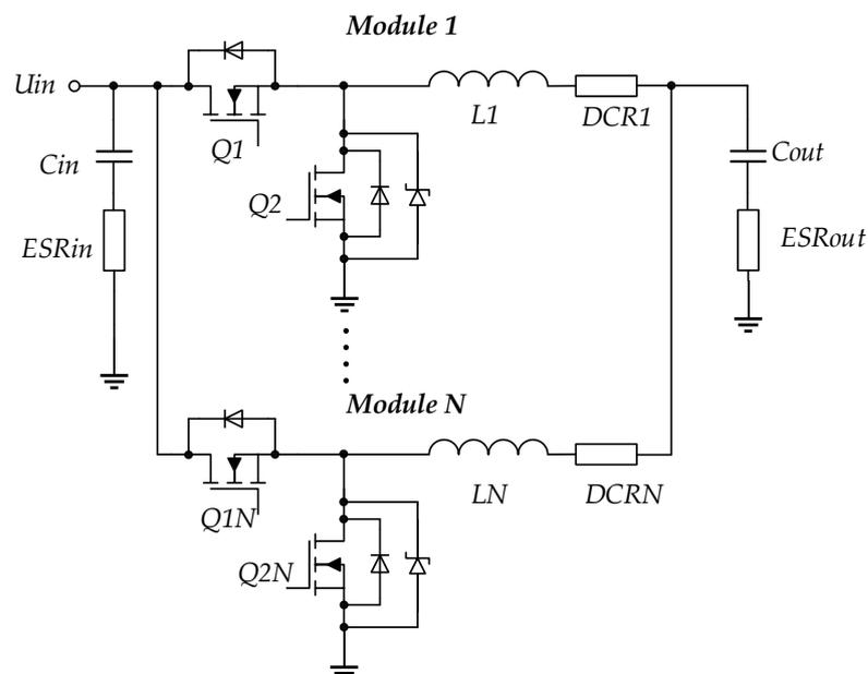
Figure 1. A multi-phase synchronous buck converter.
