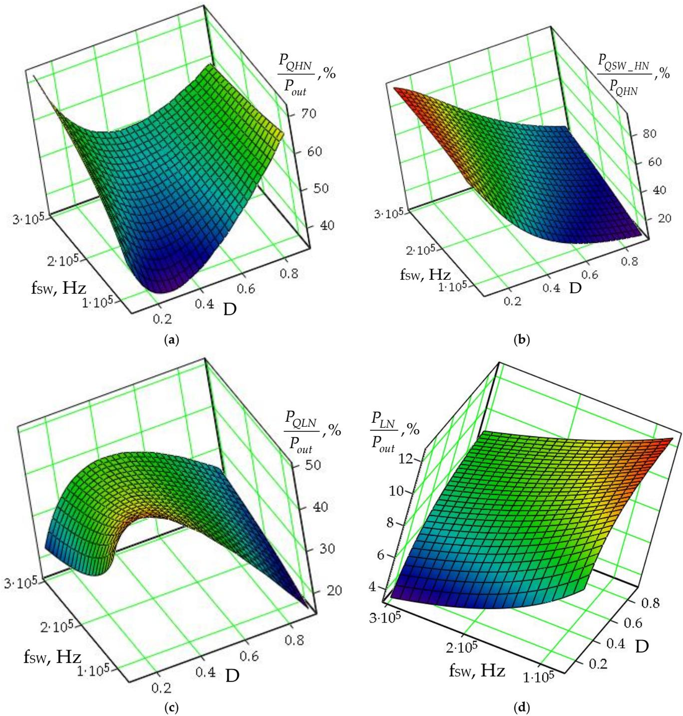
**Figure 6.** Multi-phase synchronous buck converter losses at  $U_{out} = 1.6$  V,  $I_0 = 200$  A,  $N = 8$ : (a) The total HS MOSFETs losses vs. to the total power losses  $P_{QHN}/P_{out}, \%$ ; (b) the HS MOSFETs switching losses vs. the total power losses in HS MOSFETs  $P_{QSW\_HN}/P_{QHN}, \%$ ; (c) the total LS MOSFETs losses vs. the total power losses  $P_{QLN}/P_{out}, \%$ ; (d) the inductances losses vs. the total power losses— $P_{LN}/P_{out}, \%$ .
