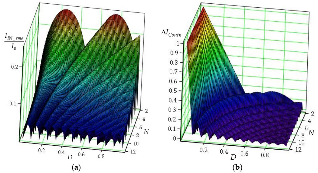
**Figure 2.** Normalized ripple currents in an N-phase converter: (a) Normalized input ripple current  $I_{IN\_rms} / I_0$ ; (b) normalized output ripple current peak-to-peak amplitude  $\Delta I_{Coutn}$ .
