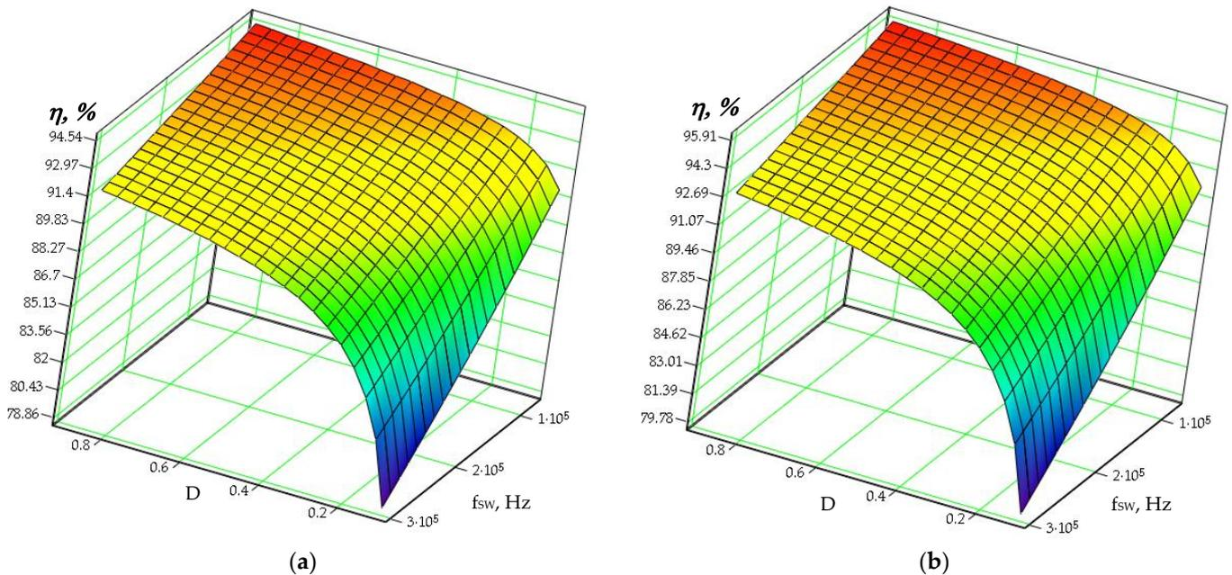
**Figure 4.** Multi-phase synchronous buck converter efficiency  $\eta(D, f_{SW})$ . (a)  $U_{out} = 1.6$  V,  $I_0 = 200$  A;  $N = 8; f_{SW} = 75$  kHz  $\div$  300 kHz;  $D = 0.1 \div 0.9$ ; (b)  $U_{out} = 1.6$  V,  $I_0 = 200$  A;  $N = 12; f_{SW} = 75$  kHz  $\div$  300 kHz;  $D = 0.1 \div 0.9$ .
