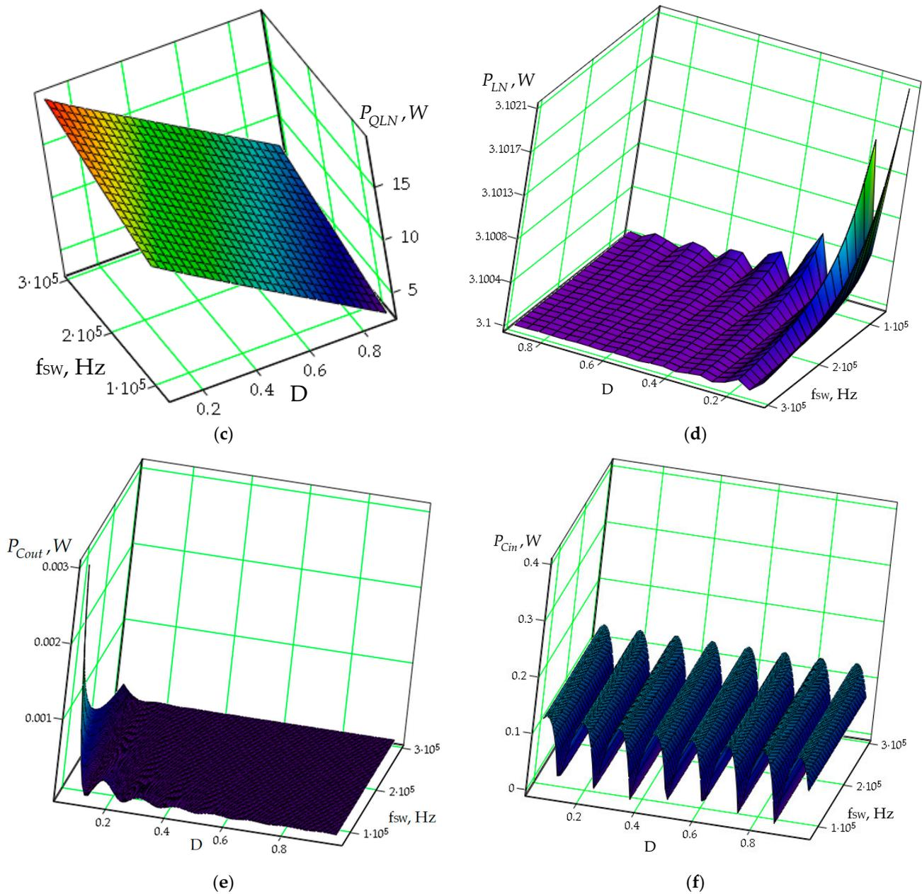
**Figure 5.** Multi-phase synchronous buck converter losses at  $N = 8$ : (a) Total power losses  $P_{out}(D, f_{sw}), W$ ; (b) total HS MOSFETs power losses  $P_{QHN}(D, f_{sw}), W$ ; (c) total LS MOSFETs power losses  $P_{QLN}(D, f_{sw}), W$ ; (d) the inductances losses  $P_{LN}(D, f_{sw}), W$ ; (e) the power losses in the output capacitor  $P_{Cout}(D, f_{sw}), W$ ; (f) power losses in the input capacitor  $P_{Cin}(D, f_{sw}), W$ .
