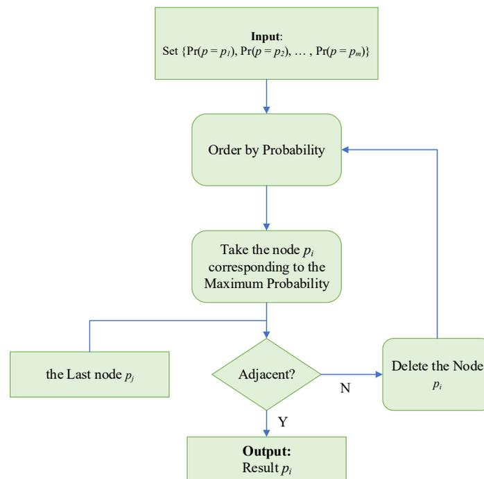
Figure 5. Error correction mechanism.
