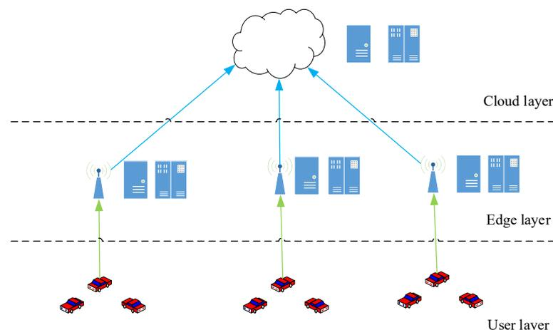
**Figure 1.** An example of vehicular edge computing.
