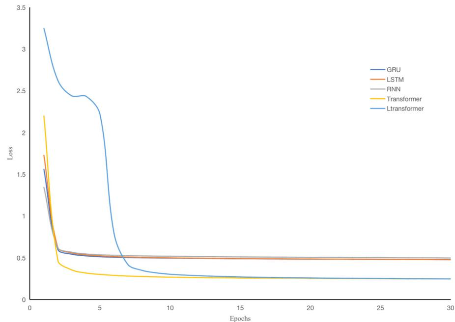
**Figure 6.** Comparison of losses of each algorithm.
