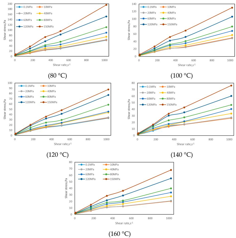
Figure 2. Variation in rheological curve with temperature in the Tianwan 1 Well.
