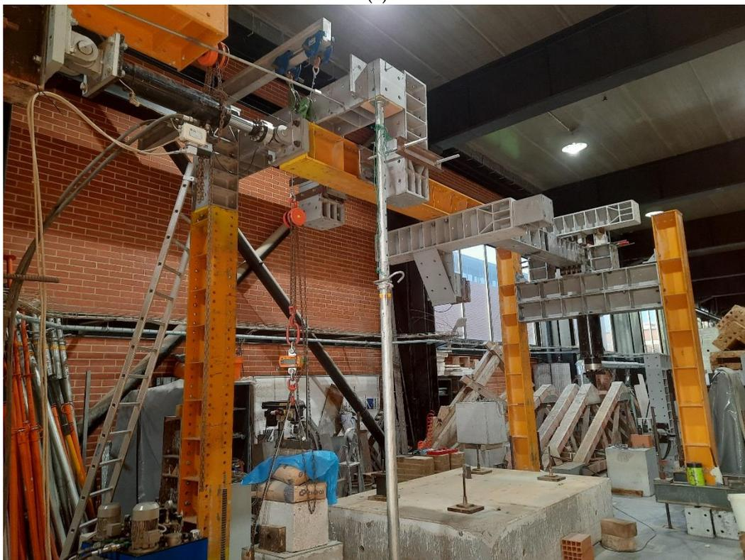
**Figure 2.** Cyclic shear test system for full-scale walls: (a) illustrating out-of-plane tests and (b) prepared for in-plane tests.
