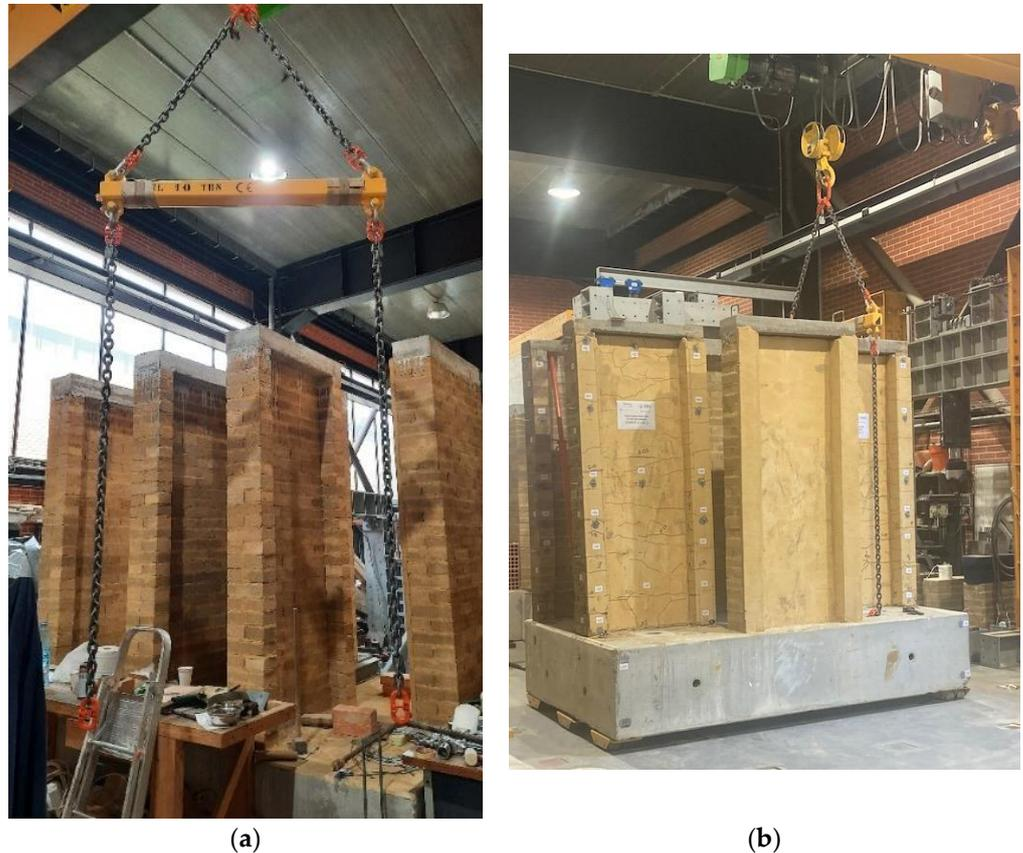
**Figure 17.** (a) Load spreader assembly. (b) Movement of the footing with specimens, with the help of roller skids, load spreader assembly, and overhead crane.
