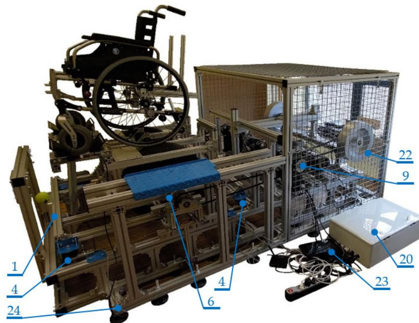
**Figure 2.** View of the wheelchair dynamometer.
