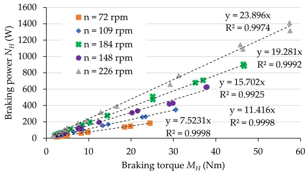
**Figure 8.** Braking power  $N_H$  as a function of braking torque  $M_H$  and rotational speed  $n$ .
