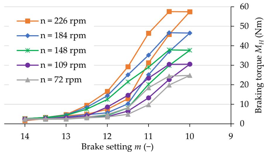
**Figure 6.** Hysteresis loops that characterize the constructed brake.
