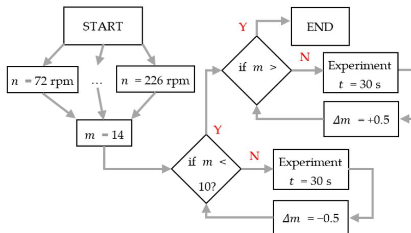
Figure 4. Measurement scheme.
