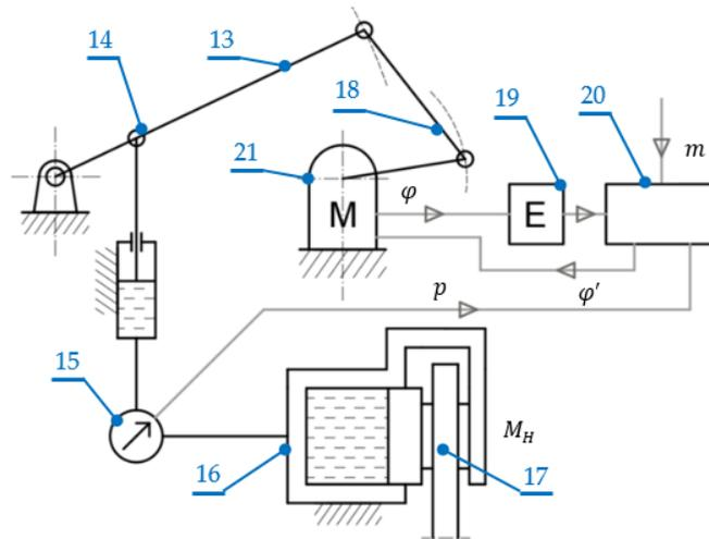
Figure 3. Design schematics for the brake control system in the wheelchair test stand.
