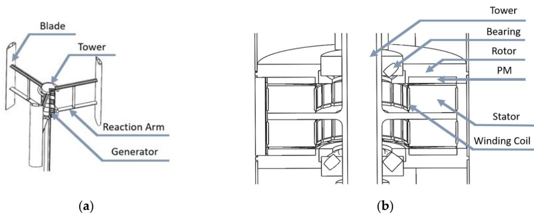
**Figure 1.** Configuration of vertical-axis wind turbine (VAWT) and outer-rotor type generator with axial-flux permanent magnet (AFPM): (a) VAWT; (b) AFPM generator.
