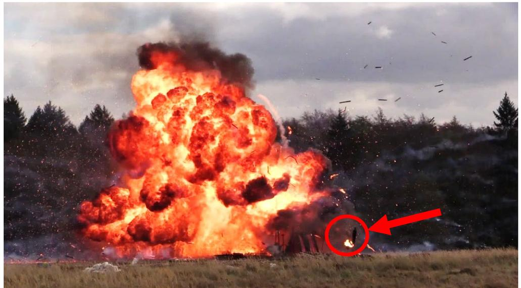
**Figure 7.** Uncontrolled destruction of acetylene cylinder (fireball).
