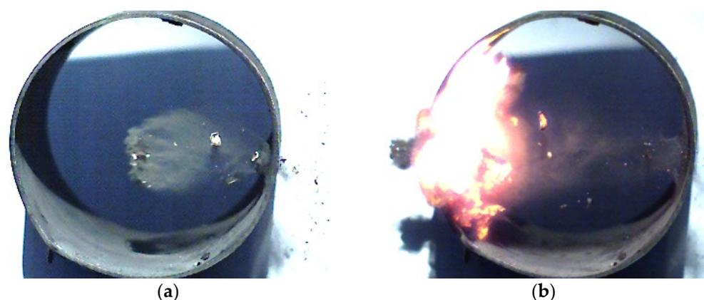
**Figure 6.** Shooting through the cylinder's cutouts: (a) shell puncture; (b) burnout of powder particles.
