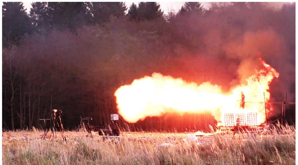
**Figure 8.** Controlled destruction of pressure cylinder (fire jet).
