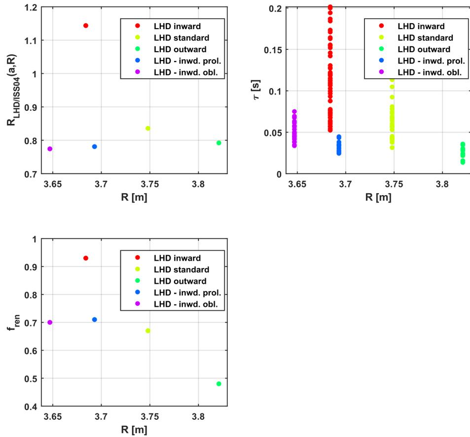
**Figure 4.** Analysis of LHD data for various optimisation levels vs. the major radius. **(Top left)** The part of the model Equation (2), which depends on major and major radius  $R_{LHD/ISS04}(a,R)$ . **(Top right)** the actual confinement time in LHD vs. the major radius. **(Bottom)** trend of  $f_{ren}$  in ISS04 vs. the major radius.
