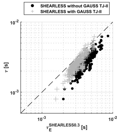
**Figure A2.** Comparison of the scaling laws with and without the exponential term for the devices without shear. In the legend of the plots, GAUSS indicates the corrective non-power law term in the scaling laws.
