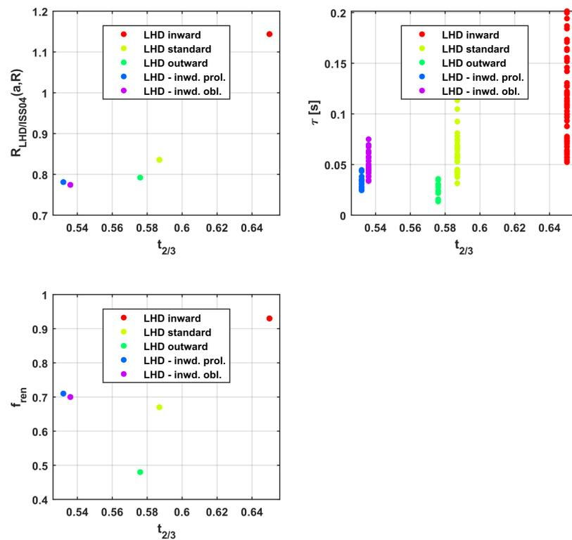
**Figure A4.** Analysis of LHD data for various optimisation levels vs. iota. **(Left)** The part of the model Equation (2), which depends on major and minor radius  $f(a,R)$ . **(Centre)** The actual confinement time in LHD vs. iota. **(Right)** Trend of  $f_{ren}$  in ISS04 vs.  $t_{2/3}$
