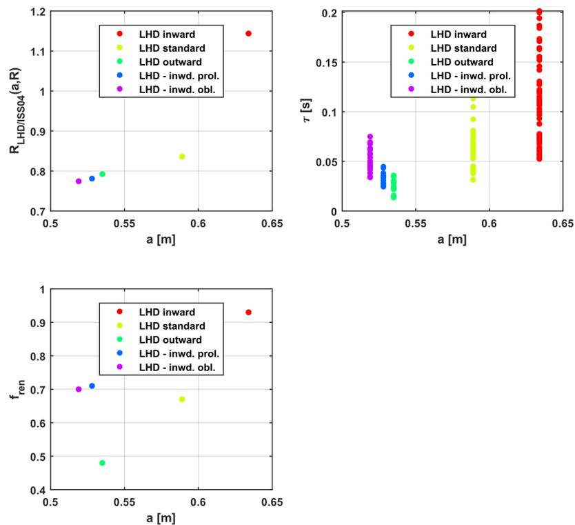
**Figure A3.** Analysis of LHD data for various optimisation levels vs. the minor radius. (Left) The part of the model Equation (2), which depends on major and minor radius  $f(a,R)$ . (Centre) The actual confinement time in LHD vs. the minor radius. (Right) Trend of  $f_{ren}$  in ISS04 vs. the minor radius.
