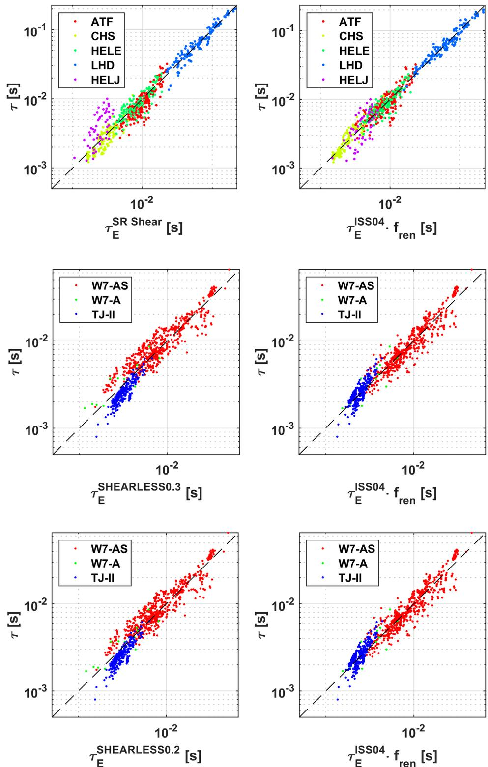
**Figure 1.** The log-log plots for the comparison of the models and the data; the experimental values of  $\tau_E$  are on the y axis and the estimates of the models on the x axis. (Left column) the models obtained with SR via GP. (Right columns) the corresponding estimates of ISS04.
