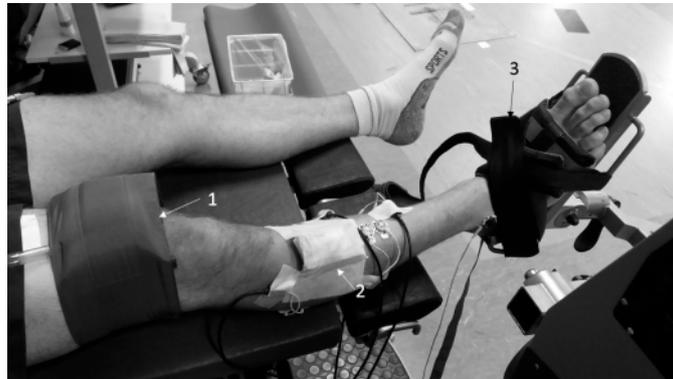
**Figure 1.** Experimental Setup. (1) Pressure cuff. (2) CW near-infrared spectroscopy device + adhesive tape. (3) Footrest including safety belts.
