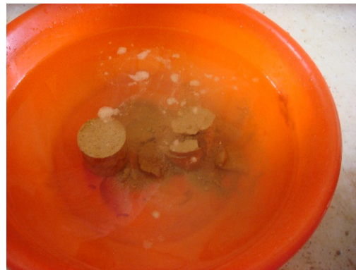
Figure 9. Soaking disintegration of modified-soil WAS (left: cement, right: quicklime).
