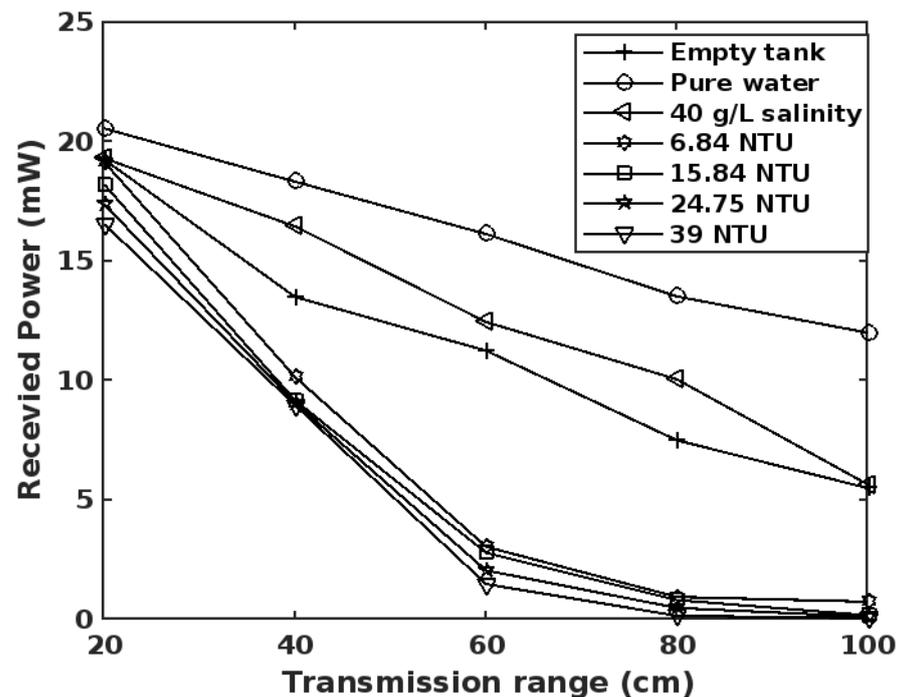
**Figure 6.** Comparison of the received power with different turbidity at different transmission distances.
