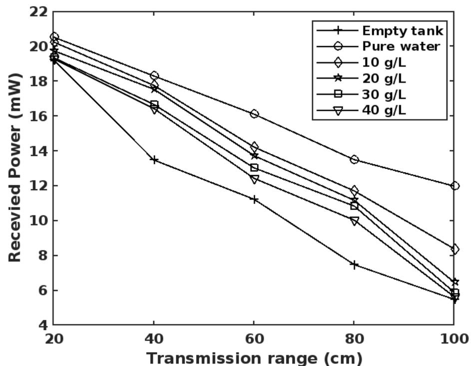
**Figure 5.** Comparison of received power with different salinity at different transmission distances.
