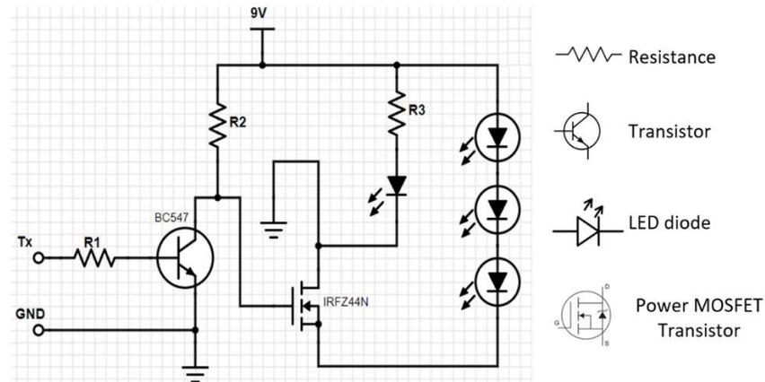
Figure 3. Light communication transmitter circuit diagram.
