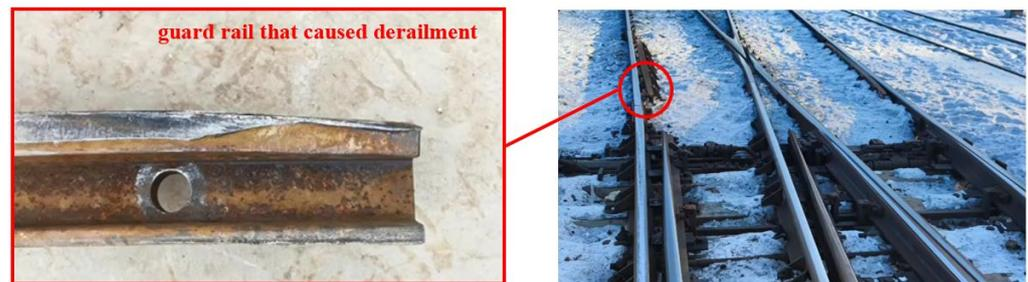
**Figure 1.** Schematic of derailment at the guardrail position in double-slip turnout.
