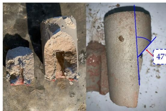
**Figure 9.** Fracture morphology of the samples damaged in slurry fracturing test [17].
