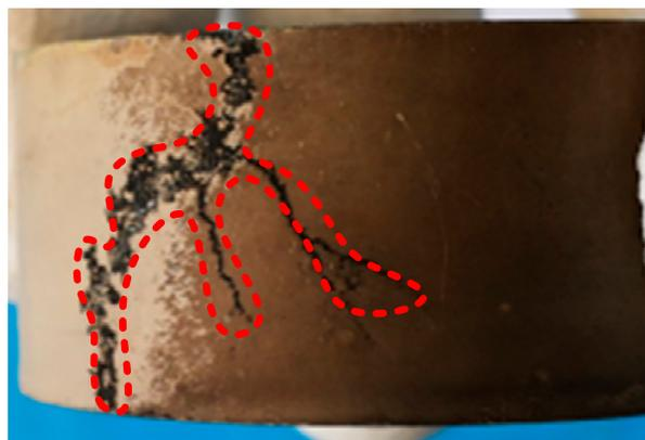
**Figure 13.** Defect valve plates.
