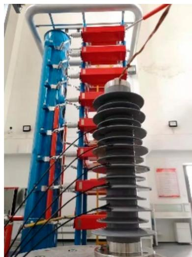
**Figure 4.** The impulse voltage generator.
