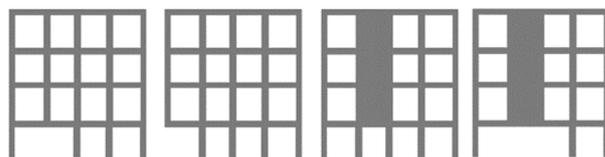
**Figure 3.** Instances of vertical irregularity.
