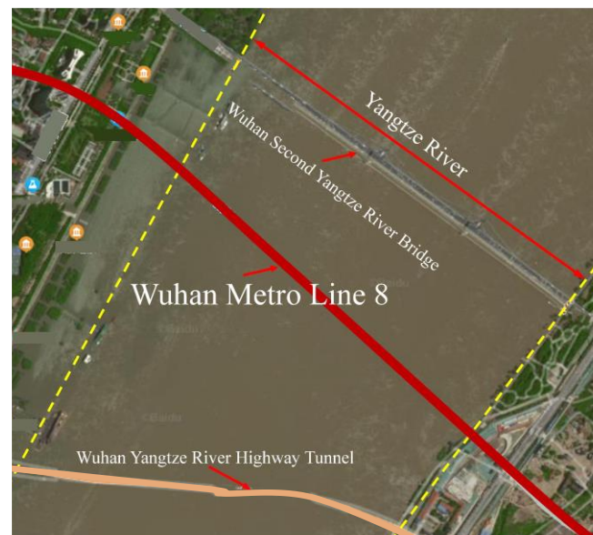
Figure 1. Plan of Wuhan Metro Line 8 crosses the Yangtze River.
