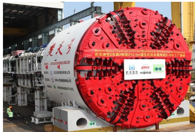
Figure 2. Herrenknecht shield machine (Chutian).
