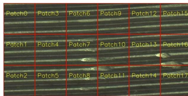
**Figure 10.** The slice patches of the panoramic screw image for the testing phase (unit: 0.03 mm/pixel).
