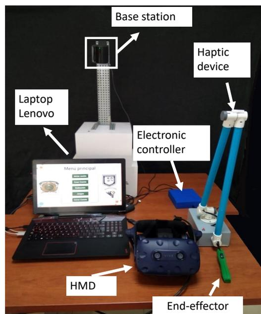
**Figure 5.** Components of the rehabilitation system.
