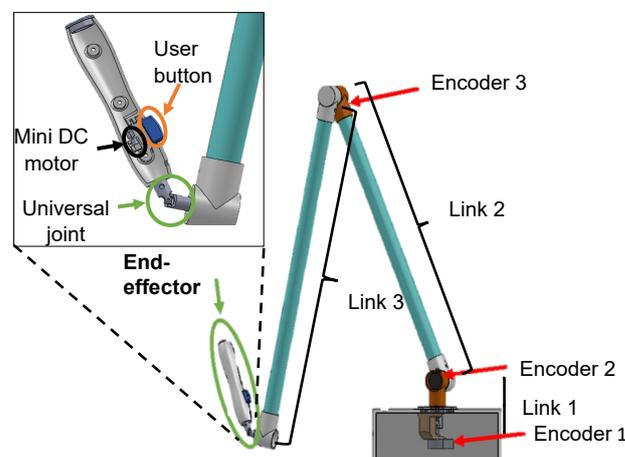
Figure 4. Haptic device and its components.
