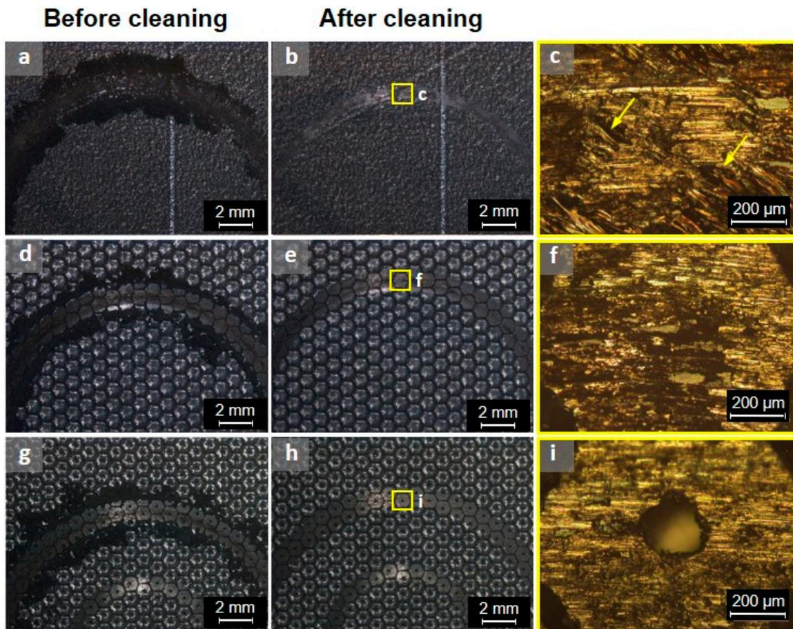
**Figure 7.** Wear tracks after 20,000 laps, R10\_N5 tests: (a–c) baseline type; (d–f) Hex\_50 type; (g–i) Hex-D\_50 type.
