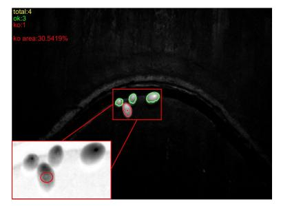
Figure 5. Example of the detection of defects in olives.
