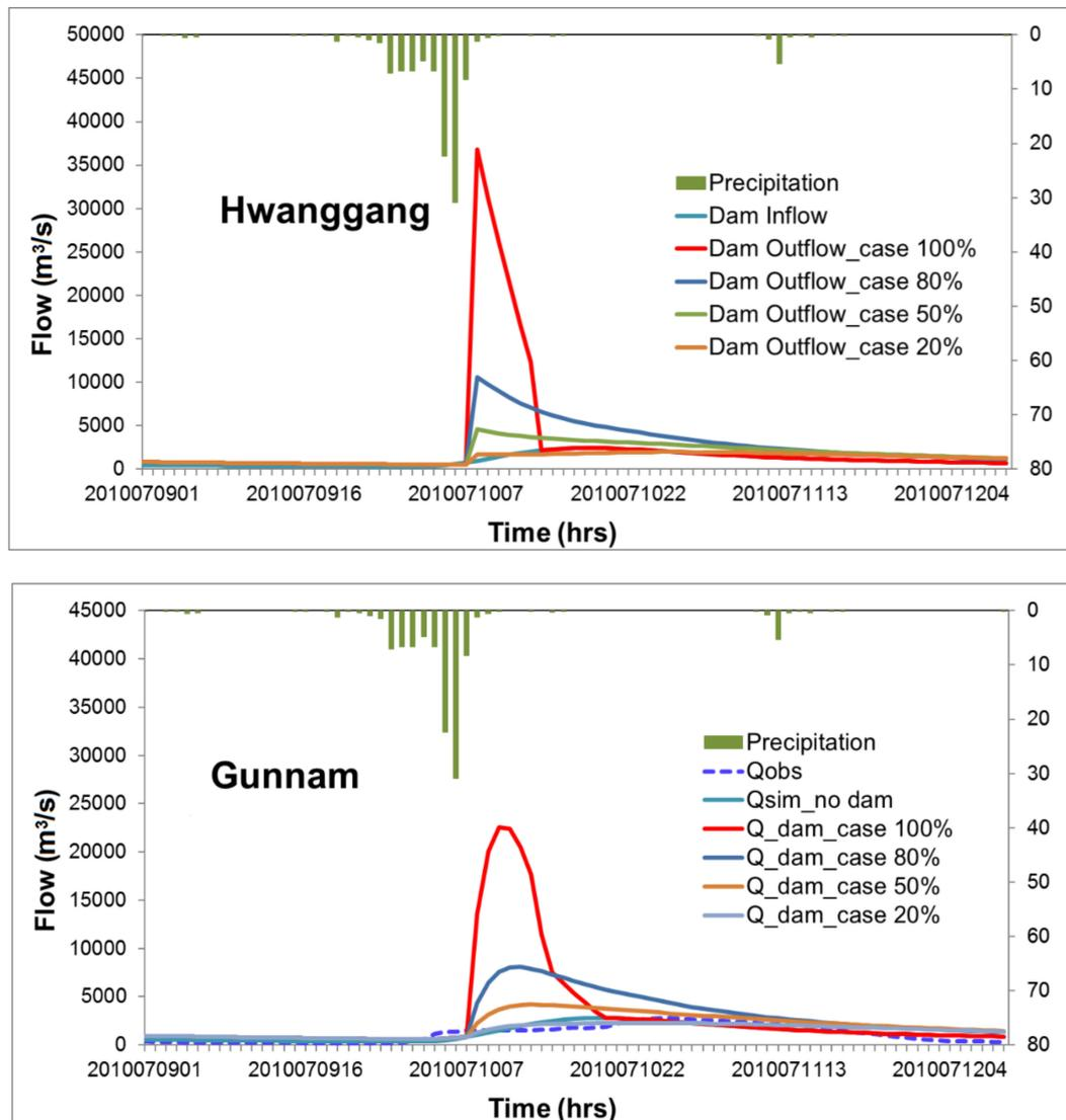
**Figure 5.** Simulated outflow at Hwanggang dam (upper) and Simulated discharge at Gunnam station (lower) in 4 dam failure scenarios.
