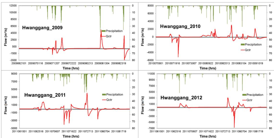
**Figure 4.** The simulated and observed discharges at Gunnam station in 4 flood events (2009, 2010, 2011, and 2012) after considering dam impact.
