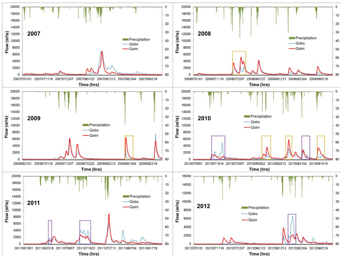
**Figure 2.** The simulated and observed discharges at Gunnam station in 6 flood events (2007, 2008, 2009, 2010, 2011, and 2012) without considering dam impact. The purple dotted line expresses the periods affected by the dam releasing water, and the orange dotted line expresses the suppositional periods affected by the dam storing water.
