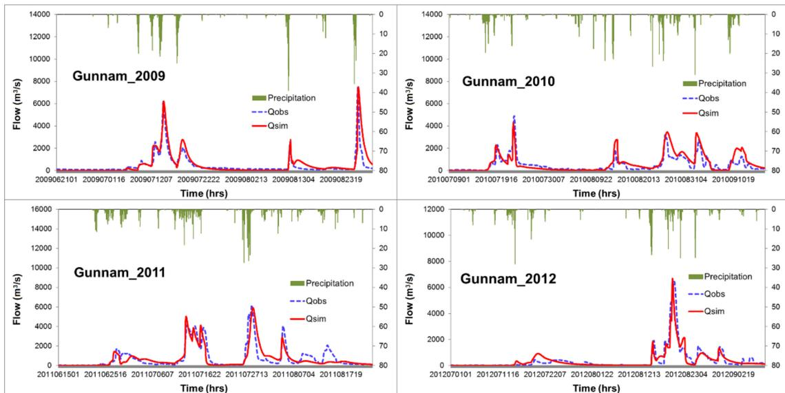
**Figure 3.** The simulated and observed discharges at Gunnam station in 4 flood events (2009, 2010, 2011, and 2012) after considering dam impact.
