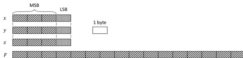
**Figure 2.** The fields and structure of an Embedding Unit (EU).
