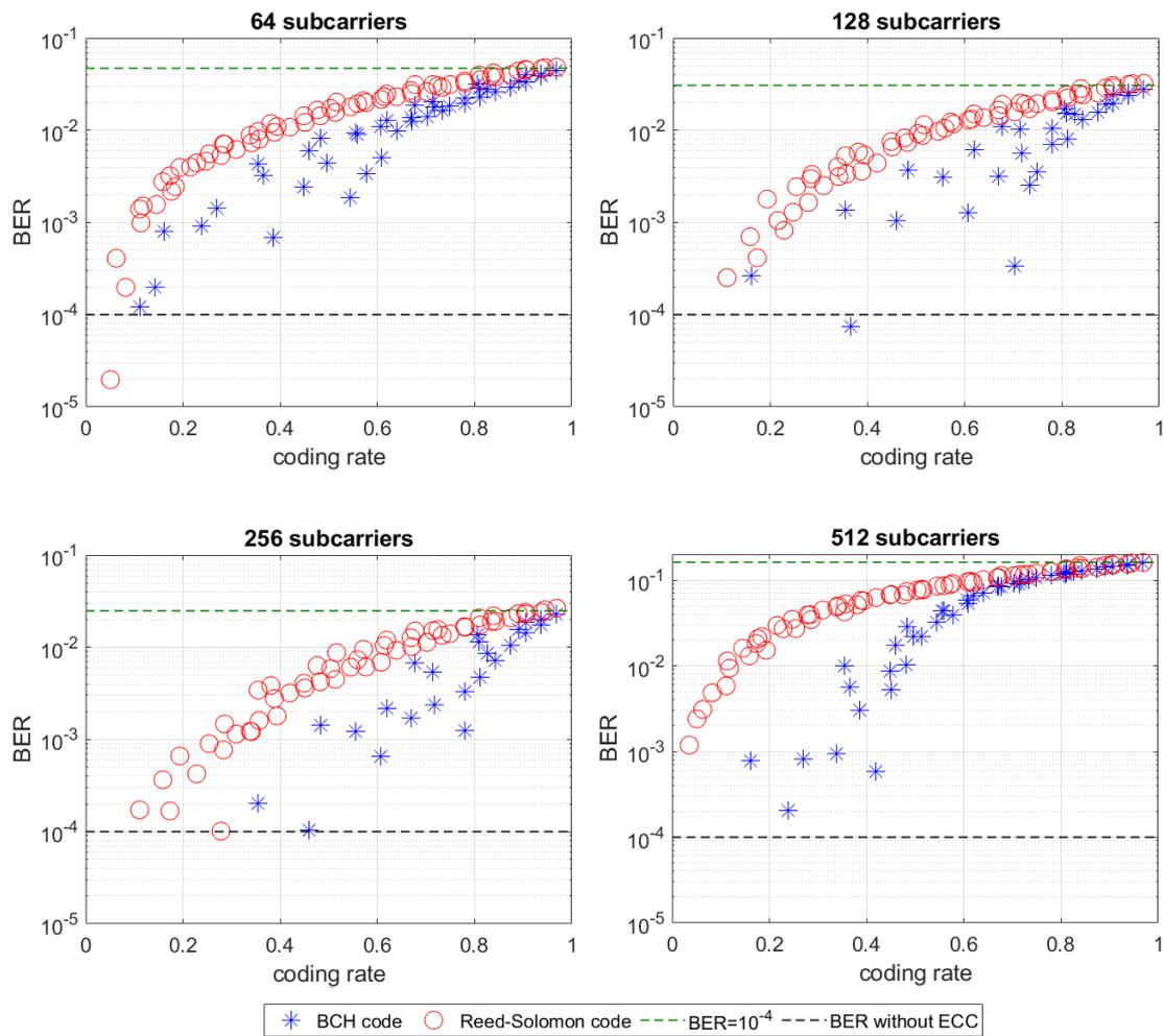
**Figure 7.** BER of OFDM data transmission as a function of ECC rate: BCH (\*) and Reed–Solomon (o); black line indicates BER equal to  $10^{-4}$ ; green line indicates BER of transmission without ECC.
