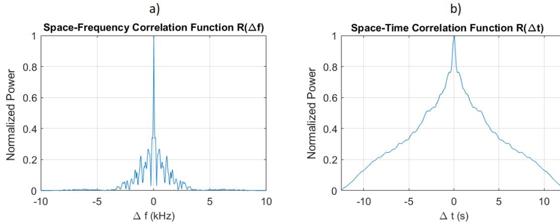
**Figure 6.** Space-frequency Correlation Function (a) and Space-Time Correlation Function (b) of the measured UAC channel at a distance of 1035 m.
