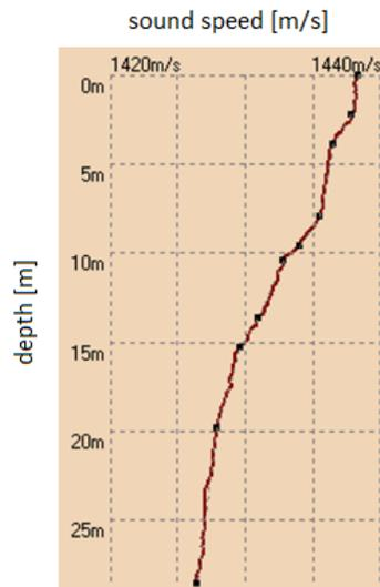
Figure 3. Sound speed profile measured during inland water experiment.
