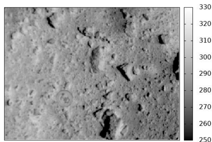
Figure 7. Thermal image of the Small Carry-on Impactor (SCI) released from Hayabusa2 spacecraft taken by TIR on 5 April 2019, at the altitude of 500 m. The shape and the attitude of the SCI was recognized in thermal images against the background of asteroid surface. A movement of SCI with its small nutation was observed in this image. The temperature scale is in Kelvin. (Image: hyb2_tir_20190405_015705_12.fit, ©JAXA).
