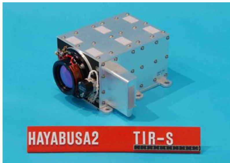
Figure 1. The flight model of the sensor unit of the thermal infrared imager TIR onboard Hayabusa2 (TIR-S). White squares on the sensor case are the Velcro tapes to attach the multi-layer insulators (MLI, the thermal blankets, not shown) which cover the sensor unit to stabilize the temperature during the operation. A baffled sunshade (not shown) is attached in front of the germanium lens to avoid insolation. The aperture of the lens is 42 mm in diameter (diameter of lens is 47 mm), and the stepping motor for the mechanical shutter is seen at the right hand of the lens. The sheet heater around the lens case is to adjust the temperature of the optics. The scale on the name plate is 10 cm long (1 cm each). (©Japan Aerospace Exploration Agency (JAXA)).
