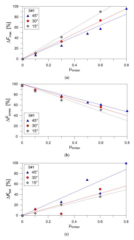
**Figure 20.** Percentage variation (Equation (4)) of performance indicators for TTC joints with inclined STSs, as a function of the timber-to-timber friction coefficient (S#1 joints under shear-compression): (a) maximum force; (b) load-bearing contribution of the STSs and (c) serviceability stiffness (ABAQUS/Explicit).
