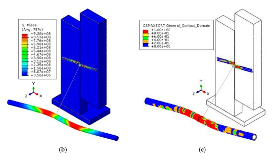
**Figure 9.** Typical damage propagation in the selected TTC joints with inclined STSs, under a standard PO setup (ABAQUS/Explicit). Example for the S#1 specimen with  $\alpha = -15^{\circ}$ , with evidence of: (a) local damage of timber (stress values in Pa), (b) yielding of screws (stress values in Pa) and (c) CZM damage parameter. Reproduced from [21] with permission from Elsevier<sup>®</sup>, Copyright license number 4895820420991, August 2020.
