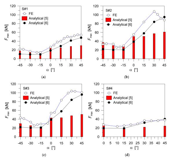
**Figure 12.** Comparison of numerical (ABAQUS/Explicit) and analytical (Eurocode 5 [5] or Tomasi et al. [6]) maximum force estimates for TTC joints with inclined STSs: (a) S#1, (b) S#2, (c) S#3 and (d) S#4 joints.
