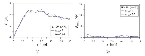
**Figure 19.** Analysis of static friction effects on the PO numerical response of TTC joints with inclined STSs. In evidence, the (**a**) vertical and (**b**) horizontal base reaction force, as a function of the measured slip (ABAQUS/Explicit).
