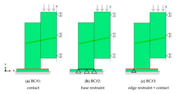
Figure 17. Analysis of boundary condition effects on the PO performance of TTC joints.
