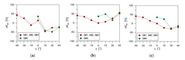
**Figure 15.** Percentage scatter of stiffness values for TTC joints with inclined STSs (Equation (5)), as obtained from the FE numerical analyses (ABAQUS/Explicit) and by literature [6]: (**a**) experimental data, (**b**) single stiffness analytical model, (**c**) double stiffness analytical model.
