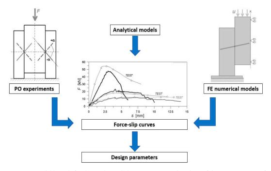
**Figure 1.** Available tools for the mechanical characterization and analysis of design parameters of timber-to-timber composite joints.
