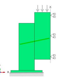
**Figure 4.** Reference FE numerical model for TTC joints with inclined STSs under a standard PO setup (S#1,  $\alpha = -15^{\circ}$ ).
