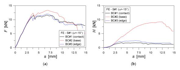
**Figure 18.** Analysis of boundary effects on the PO numerical response of TTC joints with inclined STSs. In evidence, the (**a**) vertical and (**b**) horizontal base reaction force, as a function of the measured slip for a selected TTC joint (ABAQUS/Explicit).
