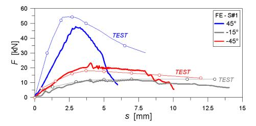
**Figure 8.** Force-slip curves of selected TTC joints with inclined STSs under a standard PO setup (ABAQUS/Explicit, S#1,  $\alpha$  = var) and corresponding experimental results (data from [6]).
