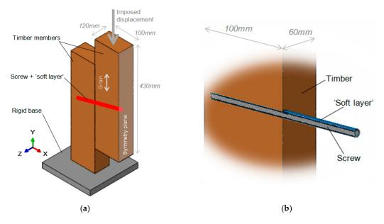
**Figure 5.** Example of (a) typical FE assembly (1/4th the S#1 geometry, with  $= -15^{\circ}$ ) and (b) detail of the STS region (ABAQUS/Explicit, hidden mesh pattern). Reproduced from [21] with permission from Elsevier<sup>®</sup>, Copyright license number 4895820420991, August 2020.
