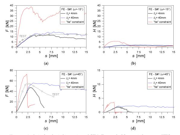
**Figure 16.** Analysis of mechanical interaction and CZM effects on the PO numerical response of TTC joints with inclined STSs (S#1). Vertical (*F*) and horizontal (*H*) reaction forces as a function of slip, for (**a**,**b**)  $\alpha$ = -15° and (**c**,**d**)  $\alpha$ = 45° (ABAQUS/Explicit).
