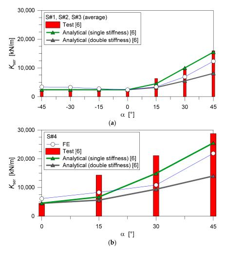
**Figure 14.** Comparison of numerical (ABAQUS/Explicit) and analytical [6] serviceability stiffness estimates for TTC joints with inclined STSs: (**a**) S#1-to-S#3 (average) or (**b**) S#4 joints.
