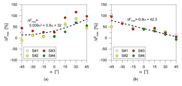
**Figure 13.** Percentage scatter of maximum force values for TTC joints with inclined STSs (Equation (5)), as obtained from the FE numerical analyses (ABAQUS/Explicit) and by literature analytical models: (**a**) Eurocode 5 [5] and (**b**) Tomasi et al. [6].
