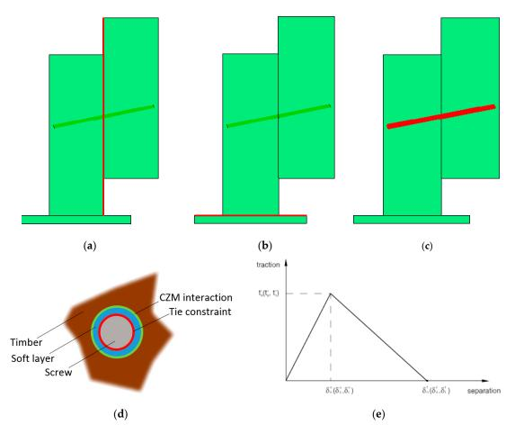
**Figure 6.** FE modelling TTC joints with inclined STSs under a standard PO setup. In evidence, the mechanical contact interactions for: (a) timber-to-timber, (b) base support and (c,d) STS details (hidden mesh pattern), with (e) traction-separation law.
