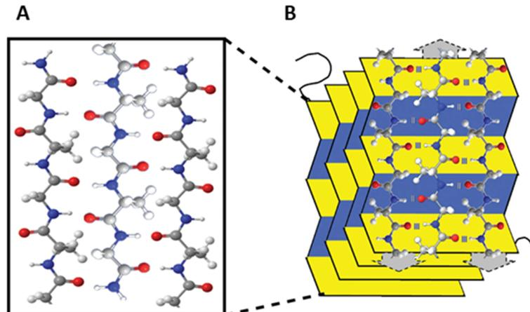
**Figure 8.** An image of a three-chain silk sequence composed of carbon (grey), nitrogen (blue), oxygen (red) and hydrogen (white) (A), and a 3-dimensional  $\beta$ -sheet of silk (B). Reproduced with permission from Cebe et al. [82] and Stewart et al. [83].
