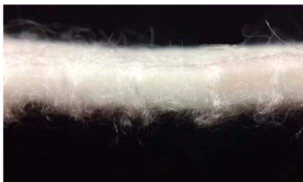
**Figure 13.** Chitosan-alginate nonwovens Composite Wound Dressings. Reproduced with permission from Gao et al. [148].
