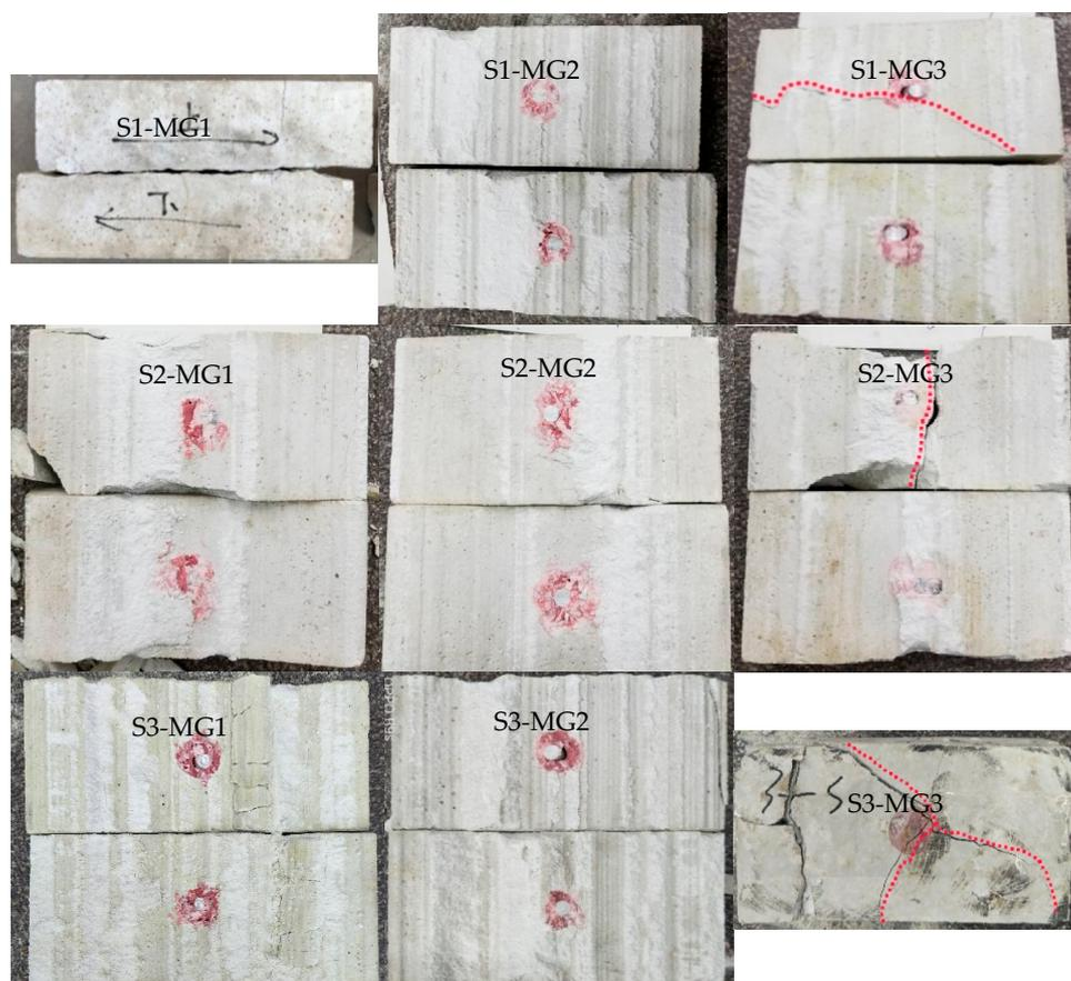
Figure 8. Experiment results of specimens with different bolts and different joint roughness.
