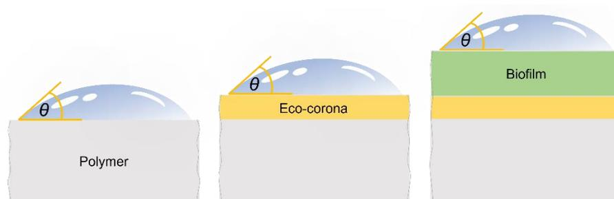
**Figure 1.** Schematic representation of surfaces resulting from the weathering of polymers: polymer surface, weathered by photooxidation, hydrolysis, or biodegradation, eco-corona layer, and biofilm layer. The outer layer is decisive for the measurement of wettability.
