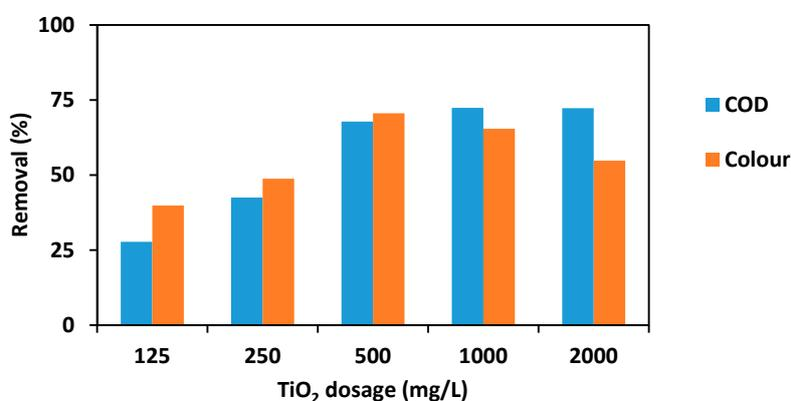
**Figure 3.** Effect of catalyst dosage on photocatalytic degradation (process conditions:  $\text{pH}$ —4, reaction time—3 h, UV light irradiation—64 W).
