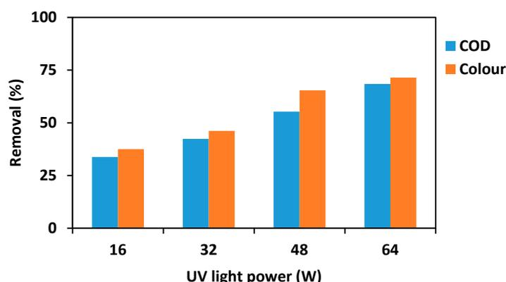
**Figure 4.** Effect of UV light irradiation power on photocatalytic degradation (process conditions: pH—4, reaction time—3 h, TiO<sub>2</sub> dosage—500 mg/L).
