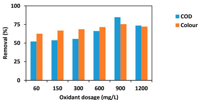
**Figure 6.** Effect of oxidant dose on photocatalytic degradation (process conditions: pH—4, reaction time—3 h, UV light irradiation—64 W, catalyst dose—500 mg/L).
