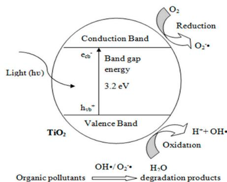
**Figure 1.** Photocatalytic mechanism for TiO<sub>2</sub> photocatalyst.
