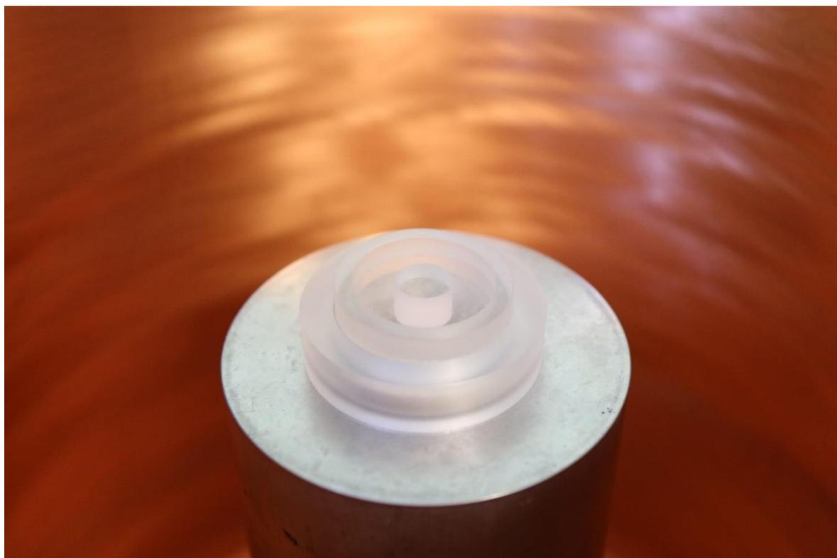
**Figure 2.** Plastic jar for the wet and dry deposition measurements placed on the top of the cap of a hyperpure germanium detectors (HPGe) detector. The dry residue (about 4 g) is uniformly distributed in a thin cylindrical shaped geometry.
