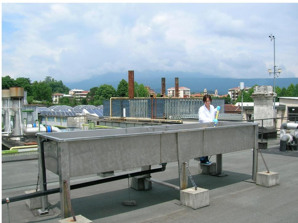
**Figure 1.** The stainless steel tank for sampling wet and dry deposition on the roof of the ARPA Piemonte building (Via Jervis, 30, Ivrea, 10015, Italy): the collection area is about 4 m<sup>2</sup> wide. The tank is emptied on a monthly basis through a tube.
