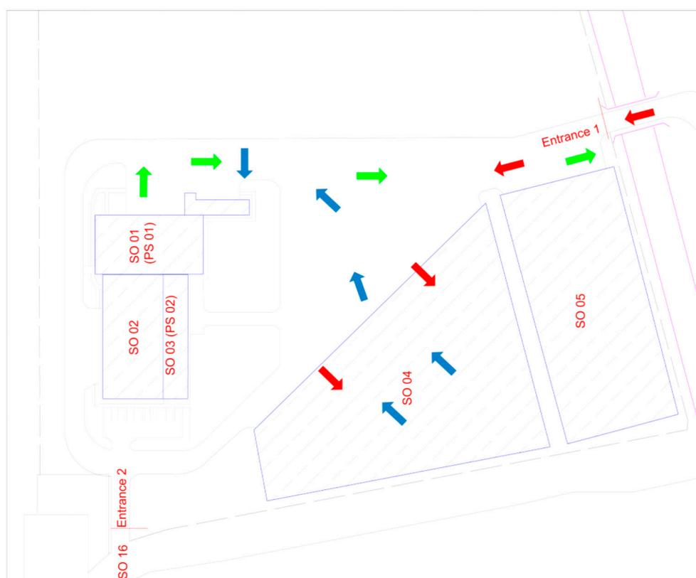
**Figure 3.** The direction of the fuel handling (source: by authors).
