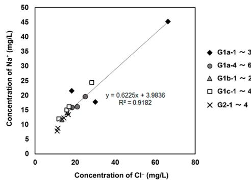
**Figure 4.** Relationship between concentrations of  $\text{Cl}^-$  and  $\text{Na}^+$  at sampling points along the Galing River.
