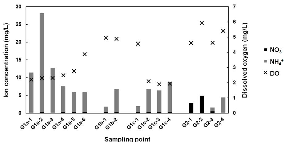
**Figure 6.** Relationship between NO<sub>3</sub><sup>-</sup>, NH<sub>4</sub><sup>+</sup>, and DO (dissolved oxygen) concentration in the Galing River.
