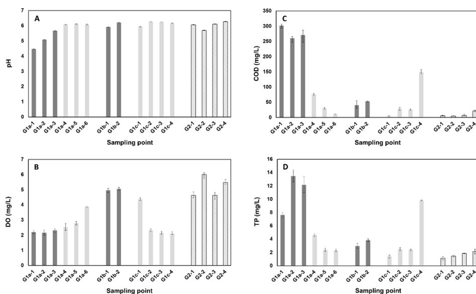
**Figure 5.** Changes in water quality indexes: (A) pH; (B) DO: Dissolved oxygen; (C) COD: Chemical oxygen demand; and (D) TP: Total phosphorus in the Galing River.
